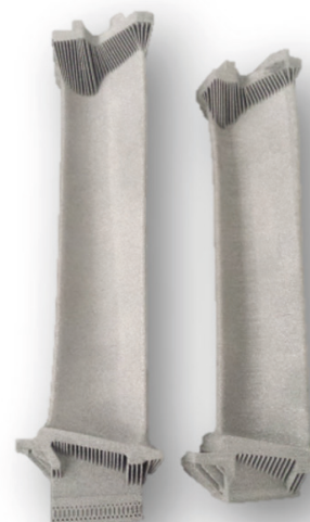
Fig.1. Example of EBM LPT blades before any HT.
