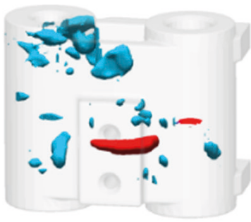
Fig. 5. Detail of predicted porosity defects due to shrinkage and air entrapment compared with X-ray analysis and destructive testing.
