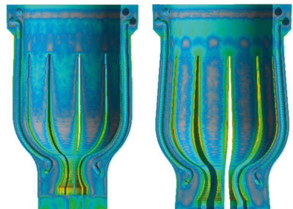
Fig. 9. Stress on the part in the as-built condition after process simulation. Left) job anchored to the platform. Right) after detachment of the part from the platform and the removal of supports.
