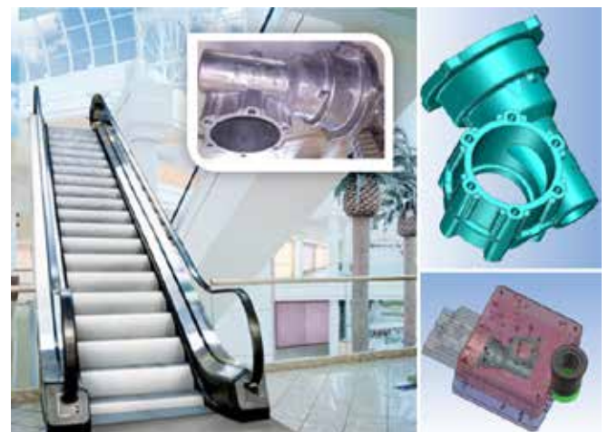
Fig. 3. High pressure die casting product: a gearmotor housing.
