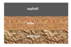
This application helps you design a flexible pavement using the approach outlined in the Highway Design Manual (6th edition) published by the California Department of Transportation (CALTRANS). Specifically, this application will determine the thickness of the subbase, base and asphalt concrete layers.
