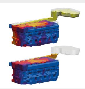
An accurate description and understanding of the processes involved in mold filling and solidification regarding the metal flow front and entrapped gases plays a decisive role in casting quality. Identifying areas where air is entrapped in the cavity during the filling process allows an optimized gating design and an effective placement of vents.
