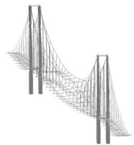
Fig. 9. Deformations of the Storebælt Bridge as the wind speed changes.
