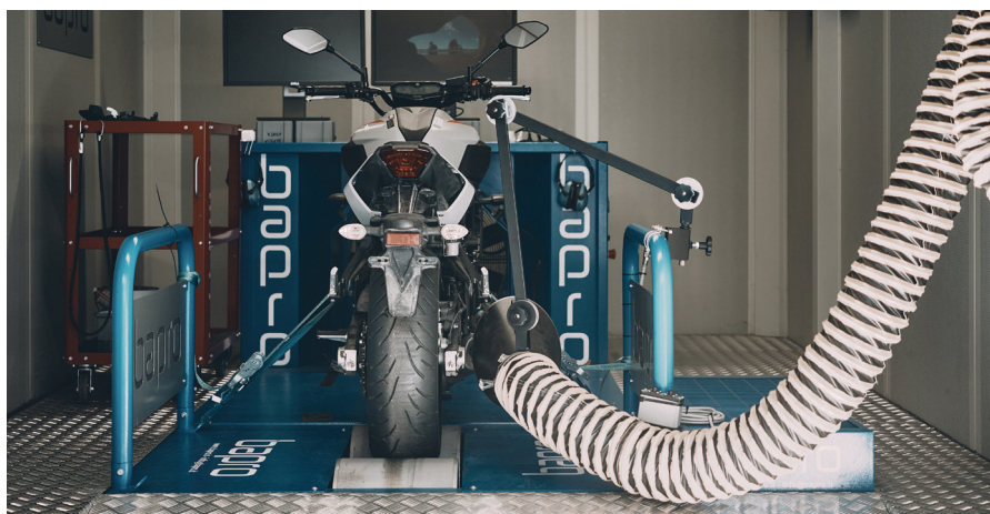
RICARDO – Dyno Roller Bench Test
