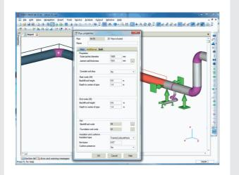
START Prof evaluates the structural responses and stresses of the different-purpose piping systems at static and cyclic loadings and performs seismic analysis. The first edition of the START Prof Software has been introduced in 1969.
