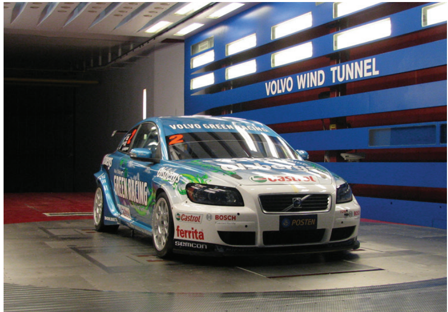
Figure 2: Polestar C30 OGR in the moving-ground Volvo wind tunnel
