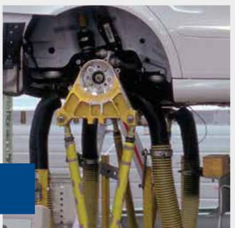
Multiaxially loaded components such as body in white (BIW), suspension components, frames or crankshafts cannot be investigated by simple methods like equivalent uni-axial loading. FEMFAT max has been developed to assess these complex loading situations in an accurate and efficient way.
