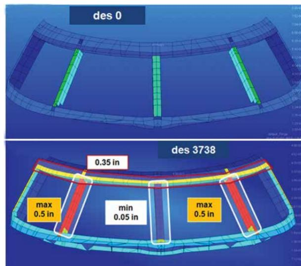
Figure 8 - FEM thicknesses - Comparison between baseline and optimum configurations
