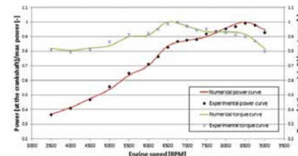
Figure 4 - Engine torque and power curves: comparison between measured and computed
