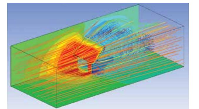
Figure 5 - Pressure Distribution and Velocity Streamlines
