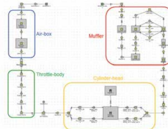
Figure 3 - Snapshot of the GT-Power engine 1D model
