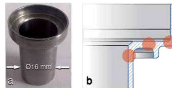
Figure 4 - a) 16 mm piston with original geometry b) Critical regions (RED)
