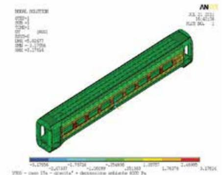
Figure 4b - displacements in y direction (mm)
