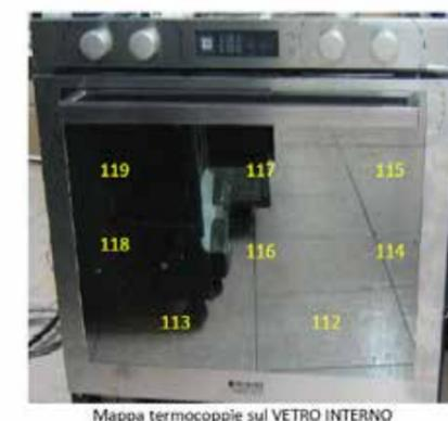
Figure 2.2.1 – Temperature measuring point on internal glass
