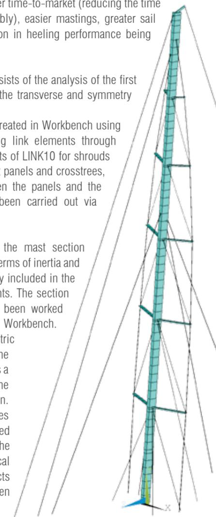
Figure 3 - Mast global buckling model
