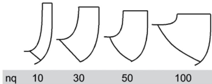
Figure 4 - Impeller form in meridional view dependent on specific speed  $n_q$
