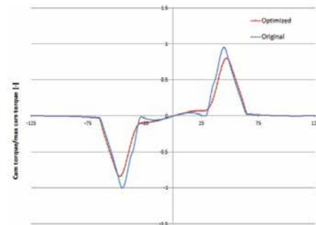
Figure 16 - Cam torque: comparison between original and optimized solution
