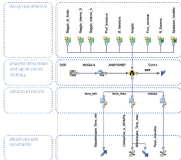
Figure 7 - modeFRONTIER design optimization workflow diagram
