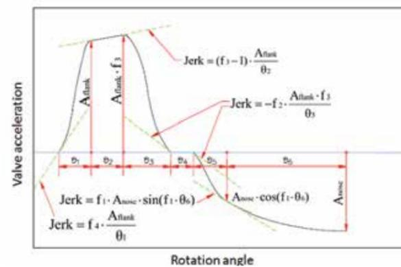
Figure 2 - Half-cam profile acceleration curve
