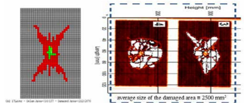
Figure 5 - Correlation between the numerical and experimental results in terms of damaged area size
