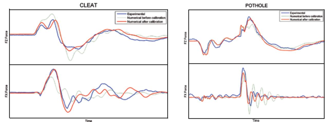
Figure 3 - Comparisons of experimental and numerical wheel forces on cleat and pothole
