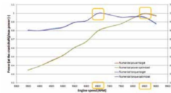
Figure 15 - Engine indicated torque and power curve: comparison between original and optimized solution (highlighted the engine speeds most significant for the analysis)
