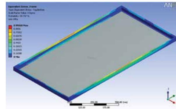
Figure 3 - von Mises stress induced by PSD
