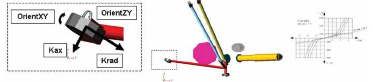
Figure 2 - Input variables: Rear suspension longitudinal arm attachment orientation and characteristics
