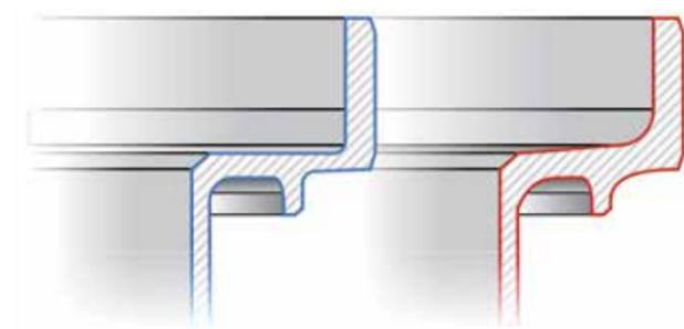
Figure 2 - Tapered Geometry (RED)
