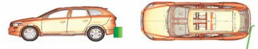
Figure 2 - Driving backwards into a fixed barrier at 15 km/h, i.e. the Allianz test, without damaging the car body is one of the toughest requirements. The figure shows the CAE model built in ANSA. This model of a full vehicle was used for verification
