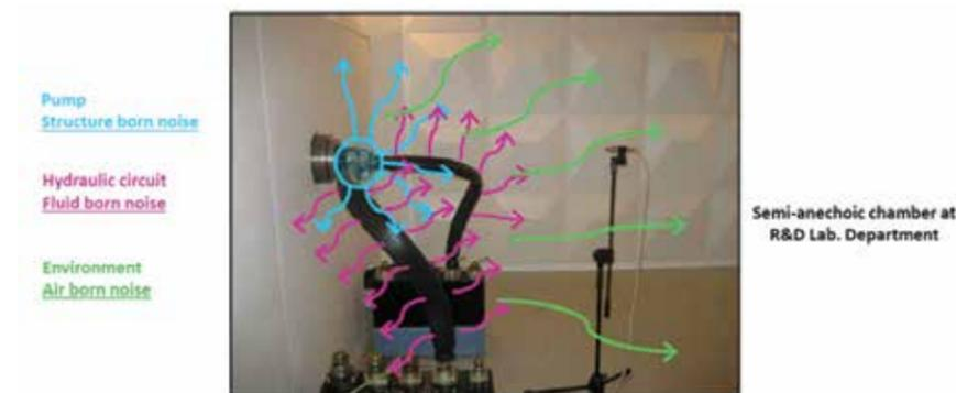
Figure 2 - Sound propagation from the pump
