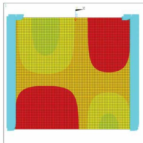
Figure 3.1.2 – Glass surface with the applied node-temperature
