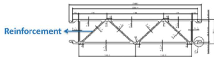
Figure 2 - Section profile of carbody
