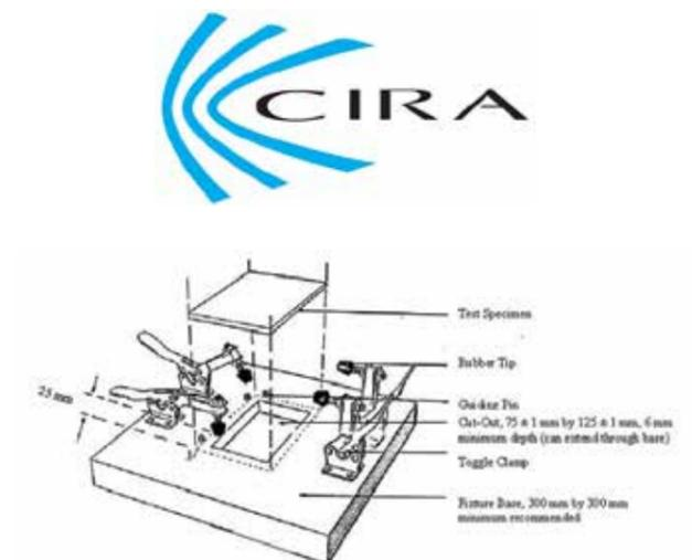
Figure 1- Impact support fixture
