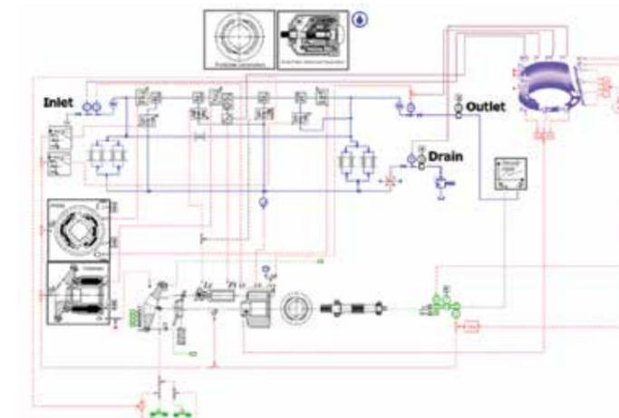
Figure 4 - AMESim model of the MVP60 pump
