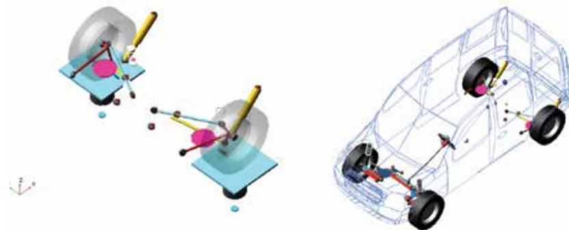
Figure 1 - Multibody Models: Rear Suspension and Full-Vehicle Handling Model - assembling Front Suspension, Steering system, Anti-roll-bar, Driveline, Engine, Rear Suspension, Body and Front & Rear Tires
