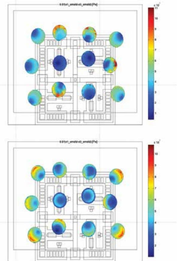
Figure 12 - Shear stress in the plane close to the PCB (upper) and the MEMS chip (lower)
