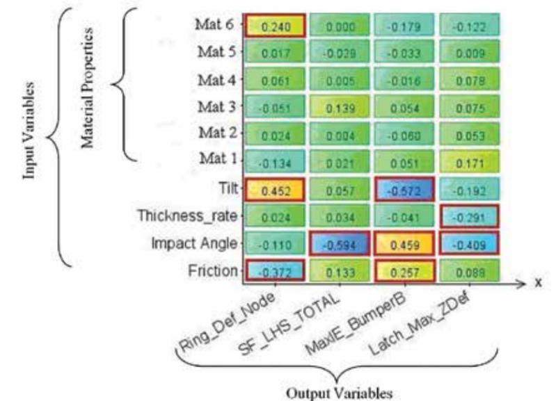
Figure 7 - Correlation between input and output variables. The variation in crashworthiness due to scatter in material properties is small if compared to the scatter in the load case variables
