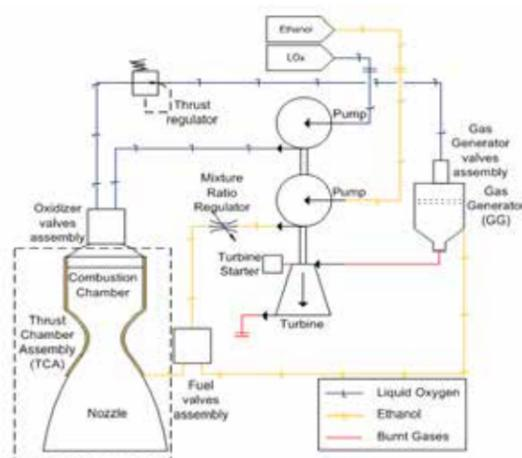
Figure 2 - L75 Engine cycle: gas generation
