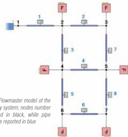
Figure 1 - Flowmaster model of the water supply system; nodes number are reported in black, while pipe numbers are reported in blue
