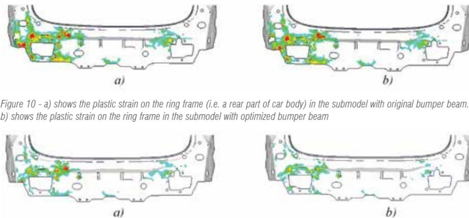
Figure 10 - a) shows the plastic strain on the ring frame (i.e. a rear part of car body) in the submodel with original bumper beam. b) shows the plastic strain on the ring frame in the submodel with optimized bumper beam
