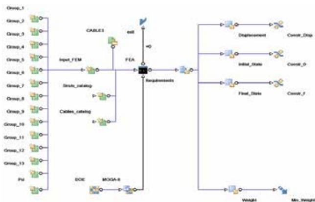
Figure 3 - Logic and data flow of the optimization process in modeFRONTIER
