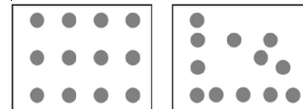
Figure 6 -- It was desirable to try out very different BGA layouts such as the example on the right, compared to the baseline design to the left
