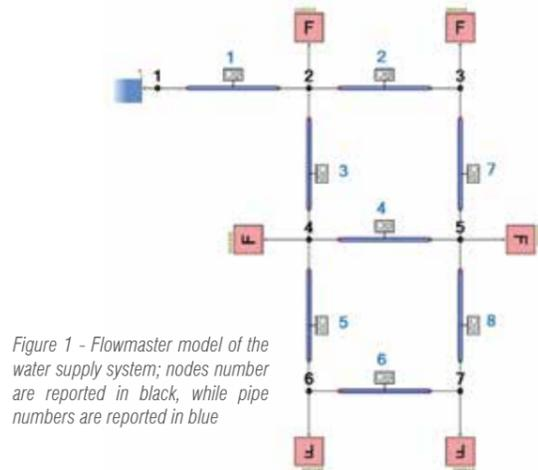
Figure 1 - Flowmaster model of the water supply system; nodes number are reported in black, while pipe numbers are reported in blue
