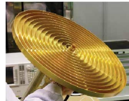
Figure 2 - Engineering Model of PDHT Isoflux Antenna with Several Series of Slots along Radial Direction
