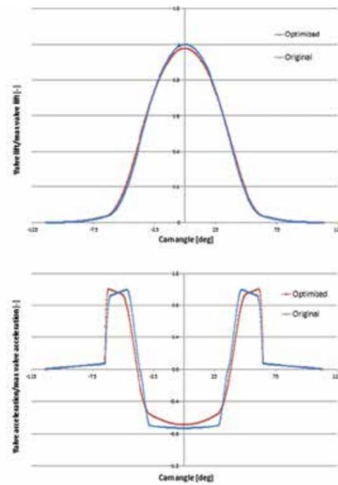
Figure 14 - Valve lift and acceleration profiles: comparison between the original and the optimized solution
