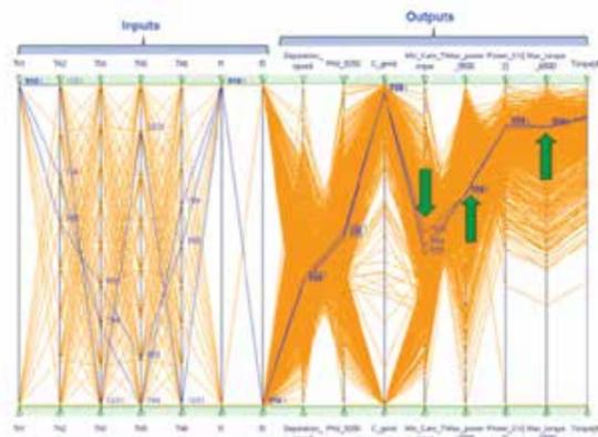
Figure 13 - Parallel coordinates chart showing the three most promising solutions (the arrows point out the objectives to minimize or maximize)
