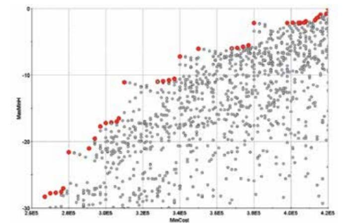
Figure 4 - Scatter plot representing the total cost and the minimum pressure level of each design; optimal designs are highlighted in red
