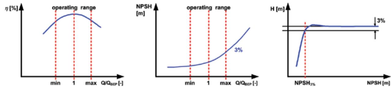
Figure 3 - left: Efficiency  $\eta$ ; centre: suction capability NPSH within the operating range of the impeller dependent on the flow rate  $Q$ ; right: NPSH3% criterion
