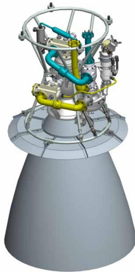
Figure 1 - L75 Engine model
