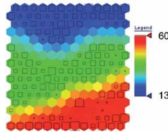
Figure 7 - Specific speed ( $n_q$ ) in the SOM with distribution of existing designs
