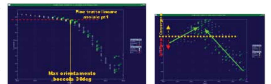
Figure 4 - Influence Scatter Charts: The left illustrates the influence of the orientation of the bushing in the X-Y plane. The right, an elasto-cinematic parameter monitored as a function of the same input variable
