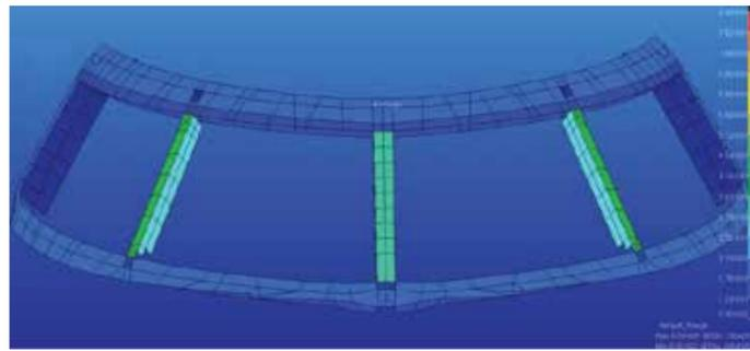
Figure 2 - Windshield GFEM properties distribution
