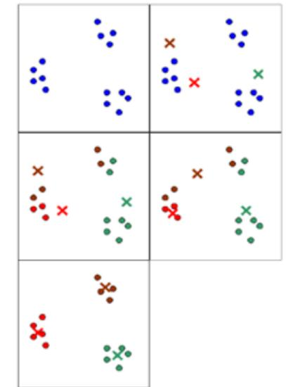
Figure 4 - Partitive Clustering step by step
