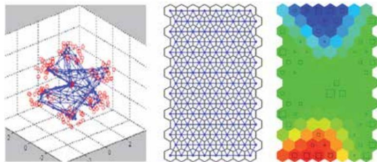
Figure 6 - Left: SOM is the blue network that adapts to real data (red points) in a X-Y-Z space, note that some nodes are far from any real point, hence the related unit will be empty. Centre: the same SOM in its 2D conventional representation: each of the nodes is a hexagonal unit. Right: each unit is colored with respect to the X-value of its prototype vector, and the square on its center represents the number of real design enclosed in the unit (see the empty units).
