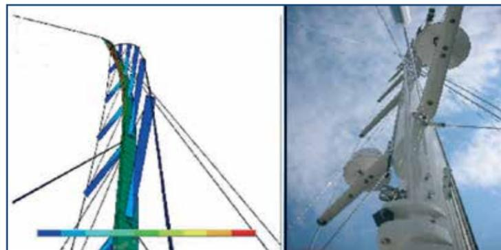
Figure 7- Preloading strain field
