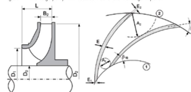
Figure 2 - Dimensions of the impeller.
