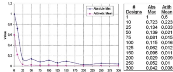
Figure 5 - Correlation between input variables approach the ideal value of zero as the number of designs grows. A maximum correlation of 0.1 between two inputs is regarded as acceptable which corresponds to a requirement of approximately 75 to 100 samples
