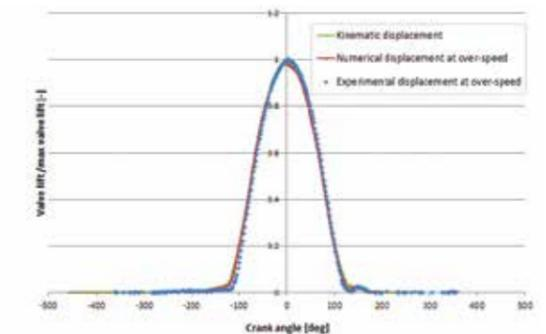
Figure 6 - Valve displacement: kinematic and dynamic profiles: comparison between measured and computed
