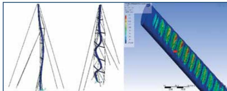
Figure 8- Shapes of global and local buckling
