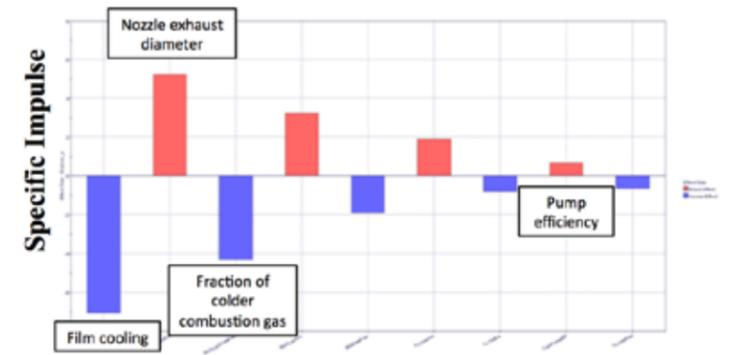
Figure 5 - Study on Specific Impulse main variables
