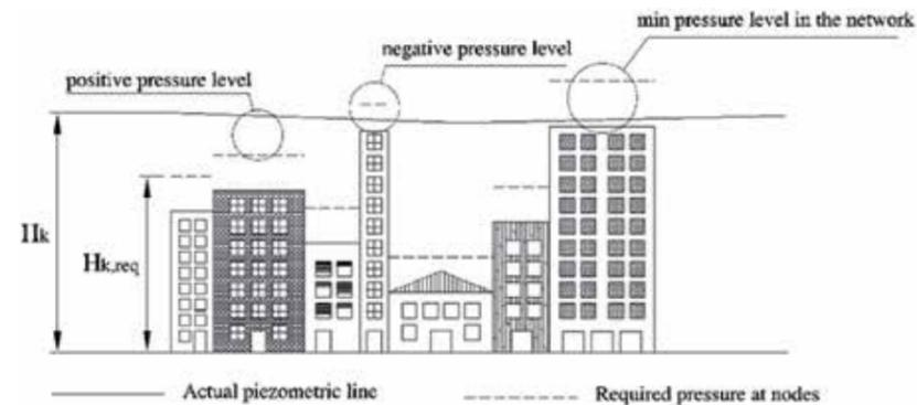
Figure 2 - Actual piezometric line ( $H_k$ ) and required pressure at nodes ( $H_{k,req}$ ) - from Nicolini (2005)
