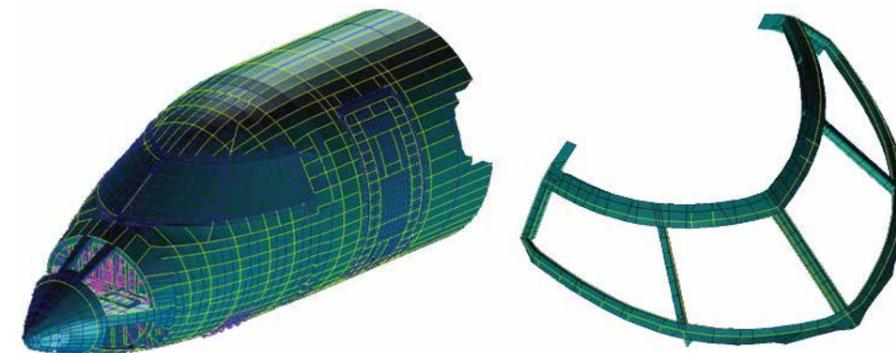
Figure 1 - GFEM: the finite element model of the Cockpit and the windshield alone
