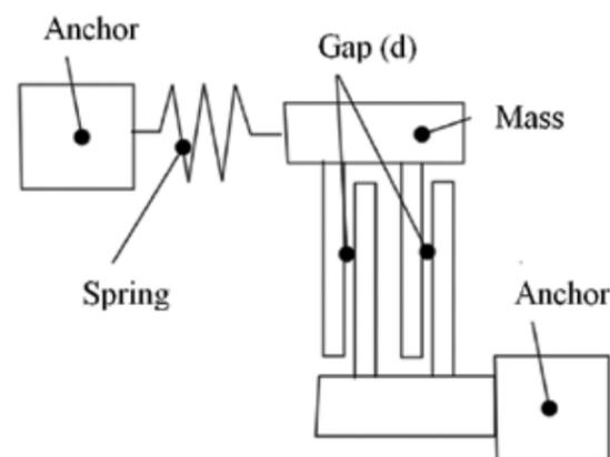
Figure 2 - A low-g accelerometer measures the change in capacitance with varying gap size. The gap, typically 1.5 to 3 μm, changes when acceleration forces move the mass
