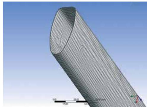
Figure 5- Mast local buckling model
