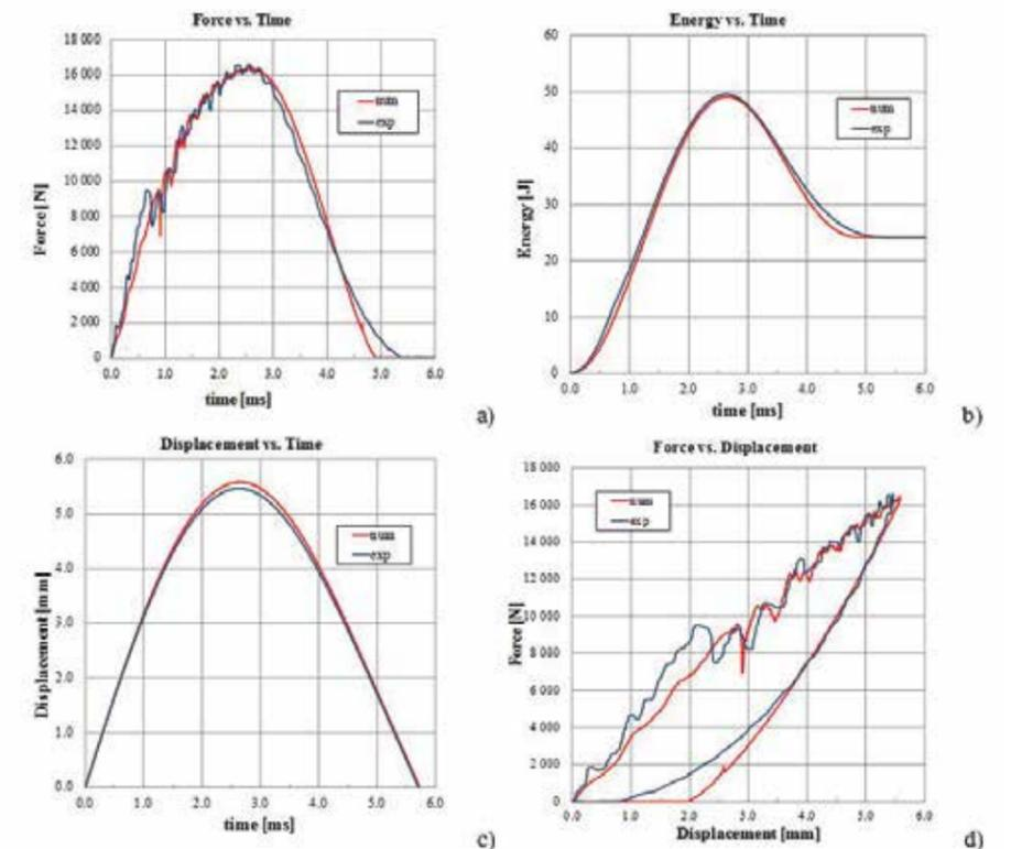
Figure 7 - Correlation between the numerical and experimental results in terms of a) contact force time histories; b) absorbed energy time histories; c) deflection time histories; d) force versus displacement trend
