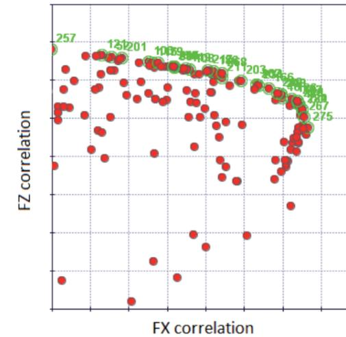
Figure 2 - Pareto frontier of numerical-experimental correlation of forces acting along X and Z directions
