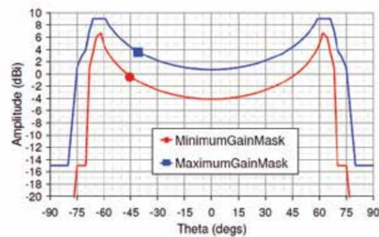
Figure 1 - Antenna Gain Requirement Mash
