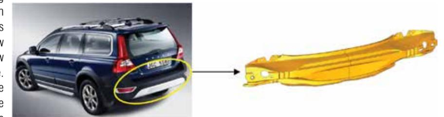
Figure 1 - Low speed crashes represent more than 70% of the crashes and combined with very high costs for repairs make robust design optimization extremely important. The study focuses on the bumper beam shown to the right
