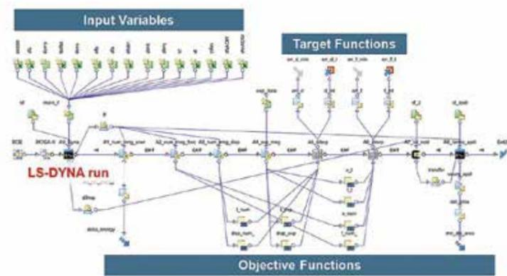
Figure 3- Sketch of the modeFRONTIER – LS-DYNA workflow
