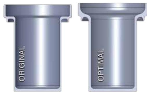
Figure 9 - Original 16 mm piston (LEFT) and Optimal piston as result of automatic optimization process
