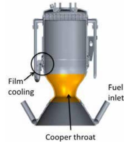
Figure 3 - Thrust Chamber Assembly (TCA) cycle design
