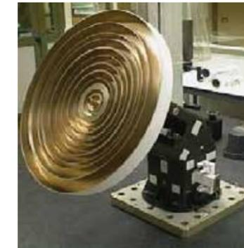
Figure 3 - Previous Flight Model of PDHT Isoflux Antenna, Corrugated Structure fed by dielectric Loaded Launcher
