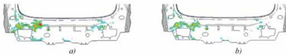
Figure 11 - a) shows the plastic strain on the ring frame in the full car model with original bumper beam. b) shows the plastic strain on the ring frame in the full car model with optimized bumper beam
