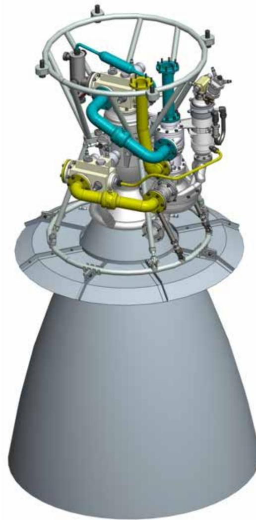
Figure 1 - L75 Engine model
