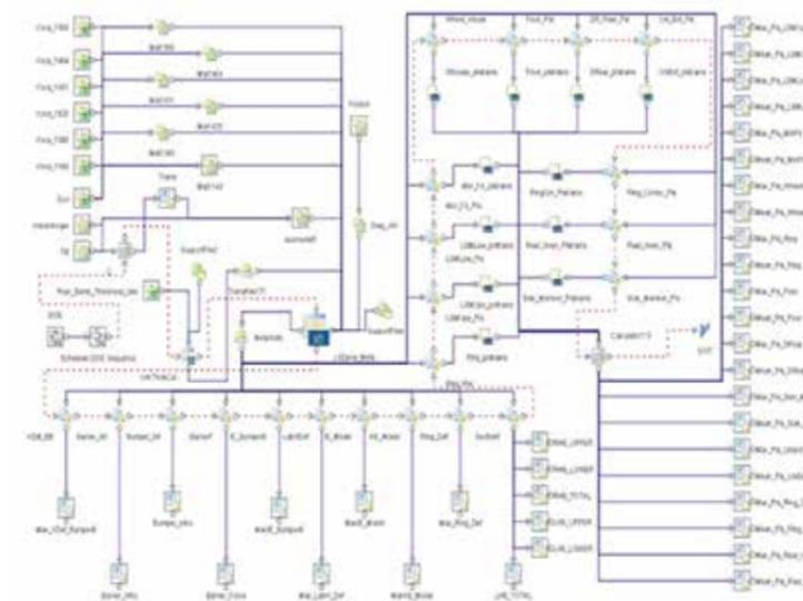
Figure 3 - modeFRONTIER was used to automate the robustness study using LS-DYNA and METApost. In order to save computational cost, a submodel instead of a full vehicle model was used for the robustness and metamodel evaluations
