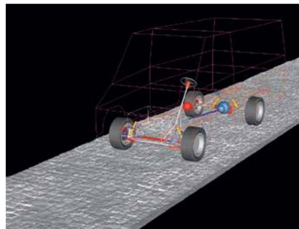
Figure 1 - Multi-body model of Iveco Daily driving on Belgian blocks test track
