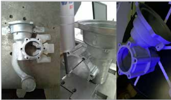
Fig. 9 – Produced die; Coordinate Measuring Machine (CMM) and optical dimensional control
