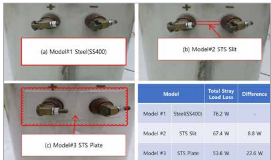
Fig. 5 – Verification test models and the results of the total stray load loss
