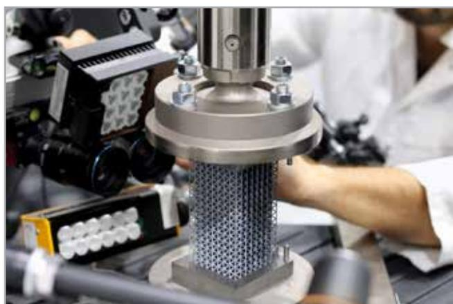
Fig. 1 – Modern structural testing often cannot rely on traditional sensors and requires more advanced techniques to provide a better understanding of deformation mechanisms (courtesy of IRT Saint-Exupéry).
