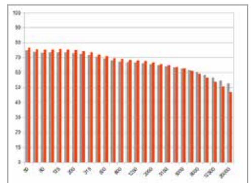
Fig. 5 – Example of background noise calibration with spectral distribution detected by MIC5: real (gray) and simulated (red)
