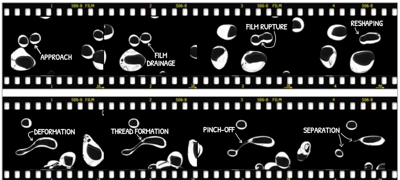
Fig. 2 - Top row shows the time sequence of a coalescence event: approach, film drainage, film rupture and reshaping, while the bottom row shows the time sequence of a breakage event: deformation, thread formation, pinch-off and separation.
