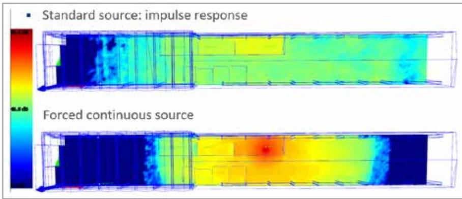
Fig. 3 – Pulse and continuous source results of the sound map [dB] inside the cabin
