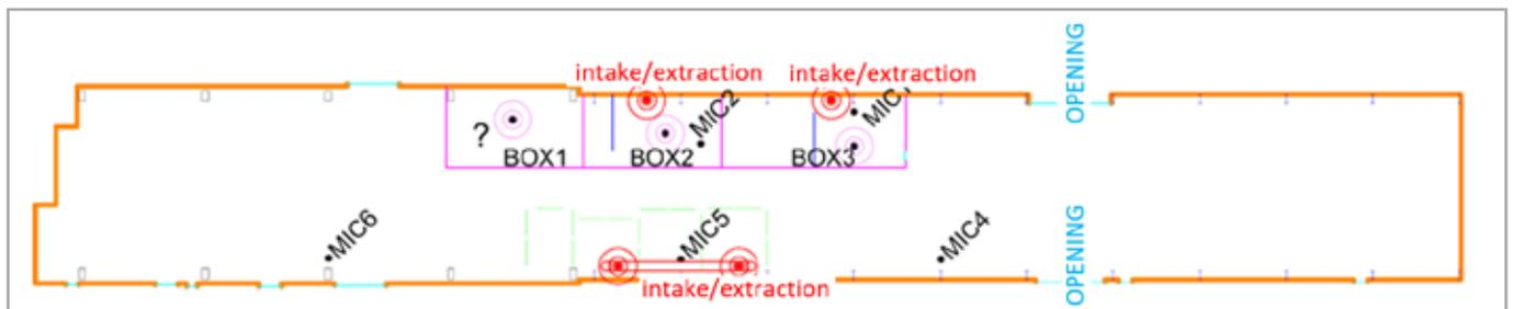
Fig. 1 – Floorplan of the mechanical workshop: cabins and microphones location
