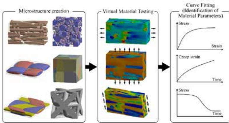
Fig. 1 – The three steps of virtual material testing in Multiscale.Sim
