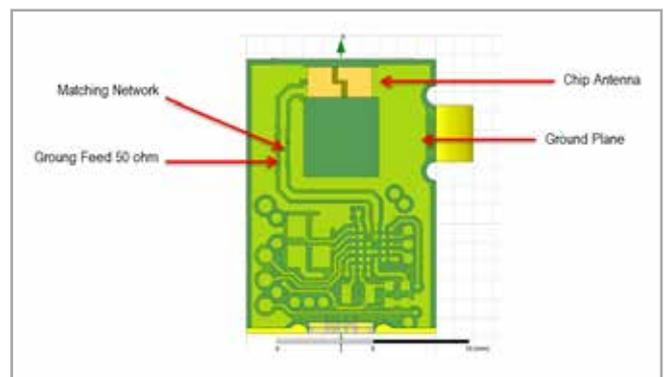
Fig. 4 – Example of PCBA with a chip antenna.
