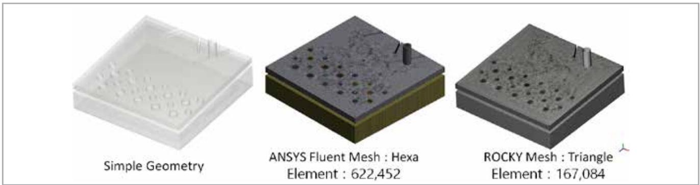
Fig. 2 – Simple geometry and mesh
