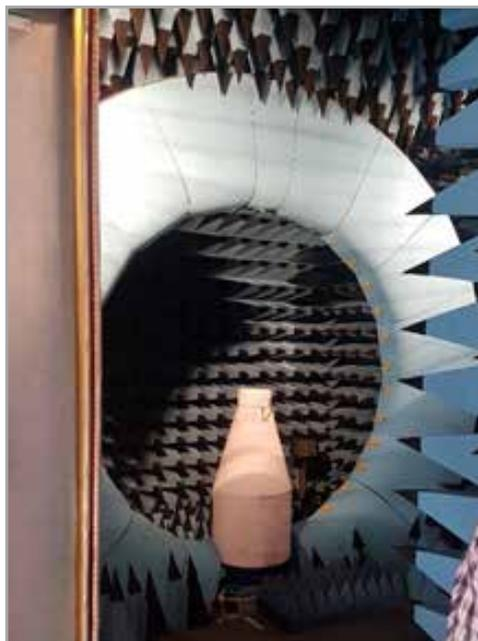
Fig. 12 – 3D radiation pattern measured in anechoic chamber
