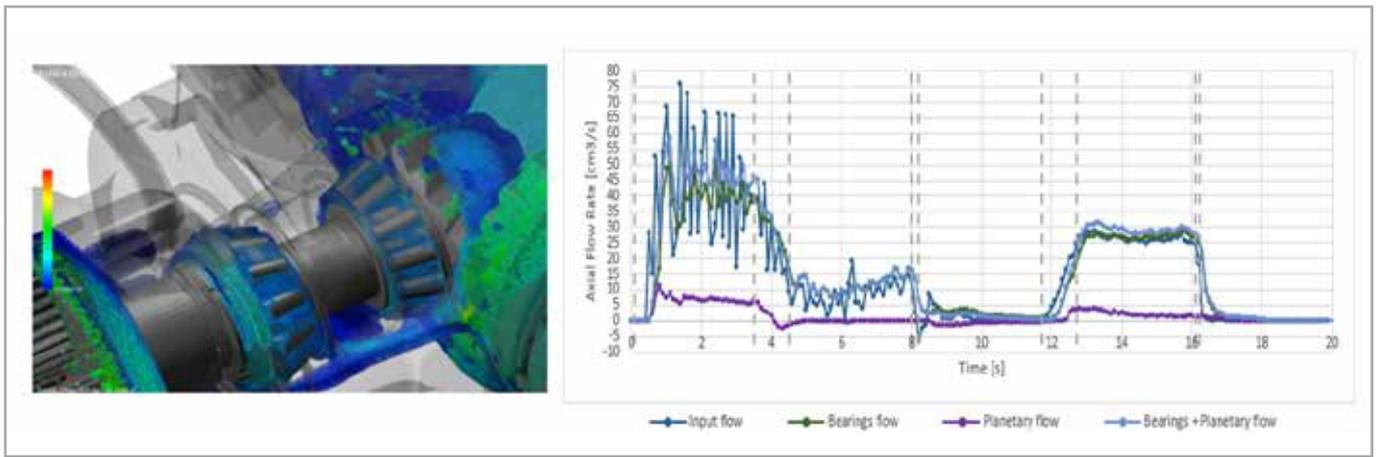
All internal components of the axle and planetary gear system were included in the model along with two variants of the housing: the first with the existing oil passage geometry and the second with some proposed optimized oil passages. Finally, the oil was modeled at its working temperature properties: the model consisted of about six million particles.
