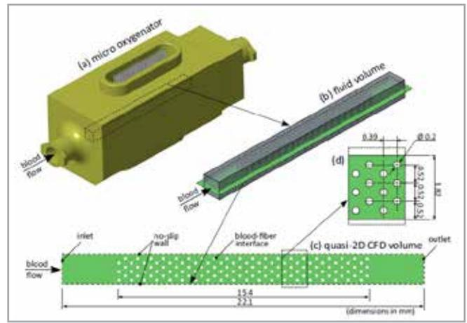
Fig.2 – Model of micro-oxygenator [2], and computational domain
