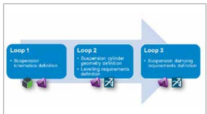
Fig. 6 - Workflow split into three loops
