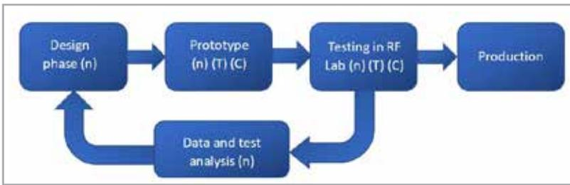
Fig. 1 – Standard Trial-and-Error Approach. Final cost of the process is calculated according to the (T)ime and (C)ost of prototyping multiplied by the number of prototyping iterations (n)
