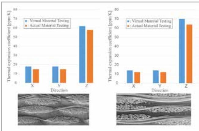
Fig. 4 – Thermal expansion coefficient measurements from actual and virtual tests
