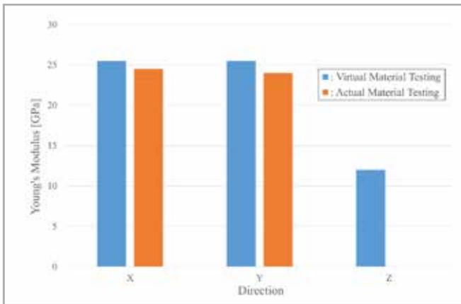
Fig. 3 – Elasticity measurements from actual and virtual tests
