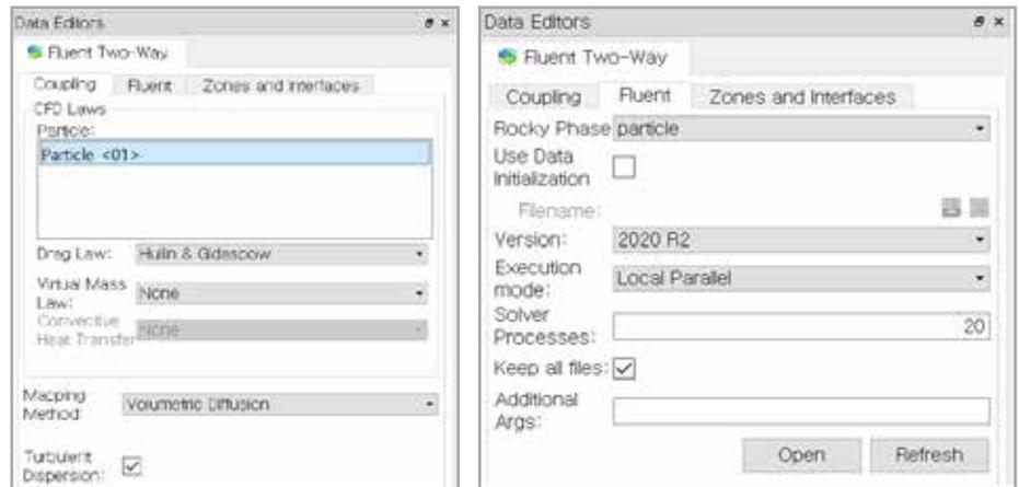
Fig. 7 – Settings for the Rocky-Ansys Fluent two-way coupling
