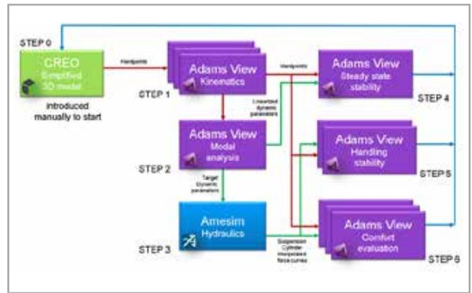
Fig. 5 - First concept of the optimization workflow
