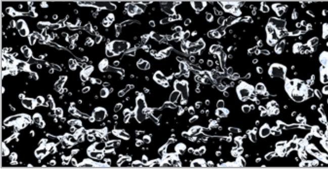
Fig. 1 – Snapshot of droplet shape (zero level of phase field) for the lowest value of surface tension considered (Weber number,  $We = 3.00$ ) and for the strongest surfactant (elasticity number,  $\beta_s = 4.00$ ).
