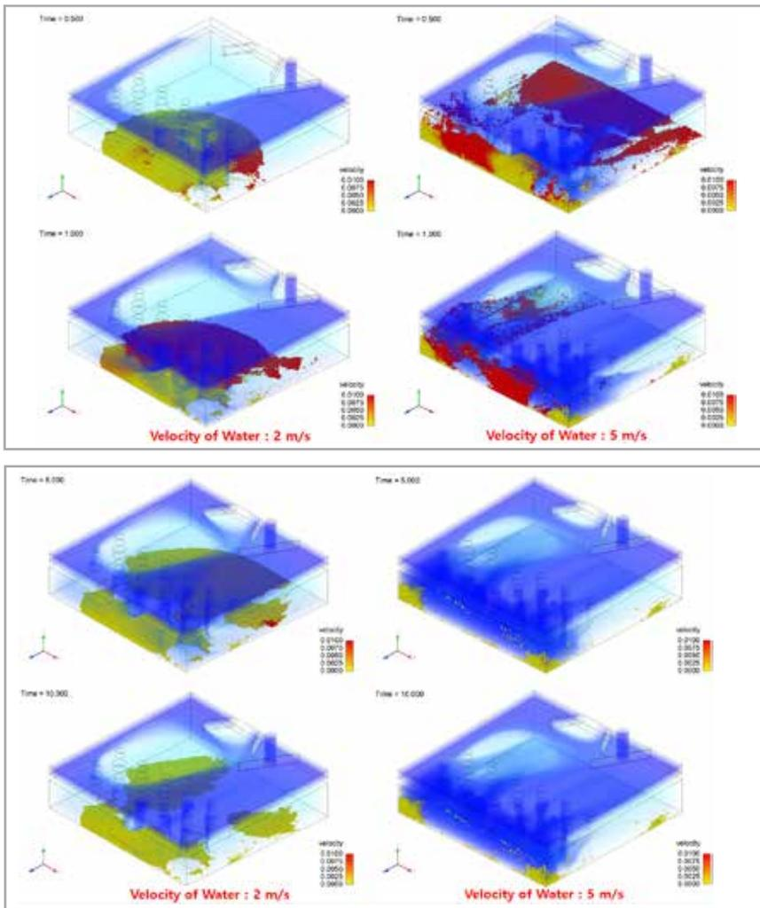
Fig. 8 – The behavior of the detergent powder according to the water flow rate
