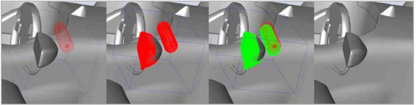
Fig. 5 – Example of RBF Morph set-up.
