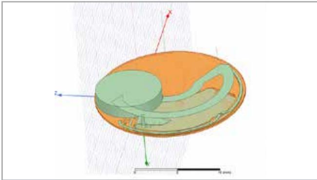
Fig. 9 – Metallic antenna derived from the battery clip.
