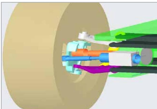
Fig. 4 - Simplified CREO model for evaluating interferences
