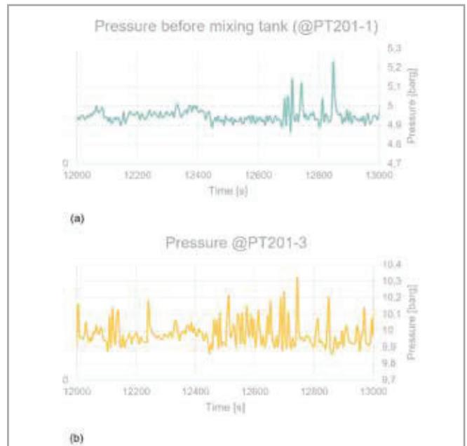
Fig. 5 – Experimental pressure variations at checkpoints.
