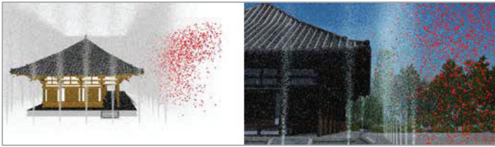
Fig. 8 – The drencher's method of preventing fire debris from reaching the building (right: CG rendering)
