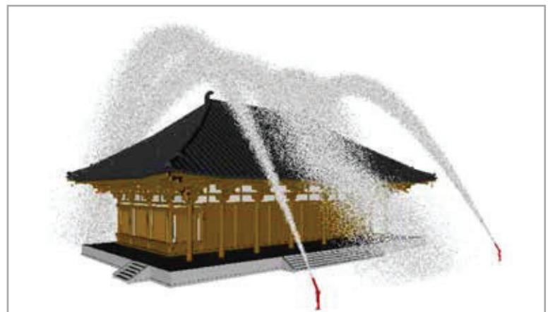
Fig. 2 – Visualization of firefighting simulation using a water discharge gun in windless conditions
