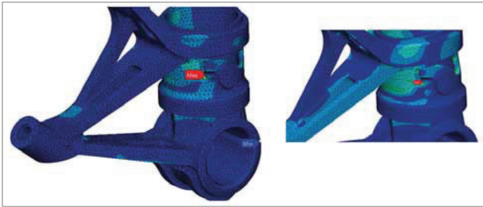
Fig. 6 - Original baseline configuration and optimized configuration after 10 iterations: maximum stress level reduced by 20.8%, increasing whole volume by 2.5%
