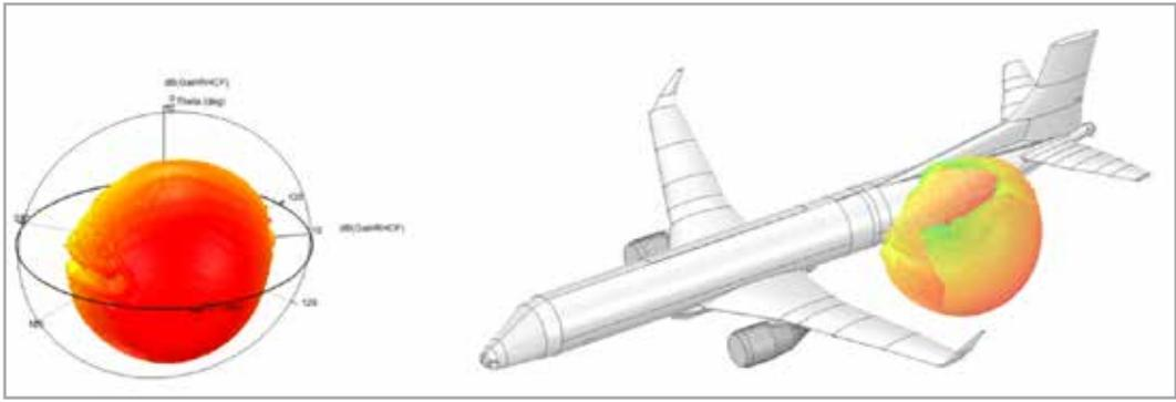
Fig. 4 – 3D Radiation pattern of the installed antenna at 3 GHz
