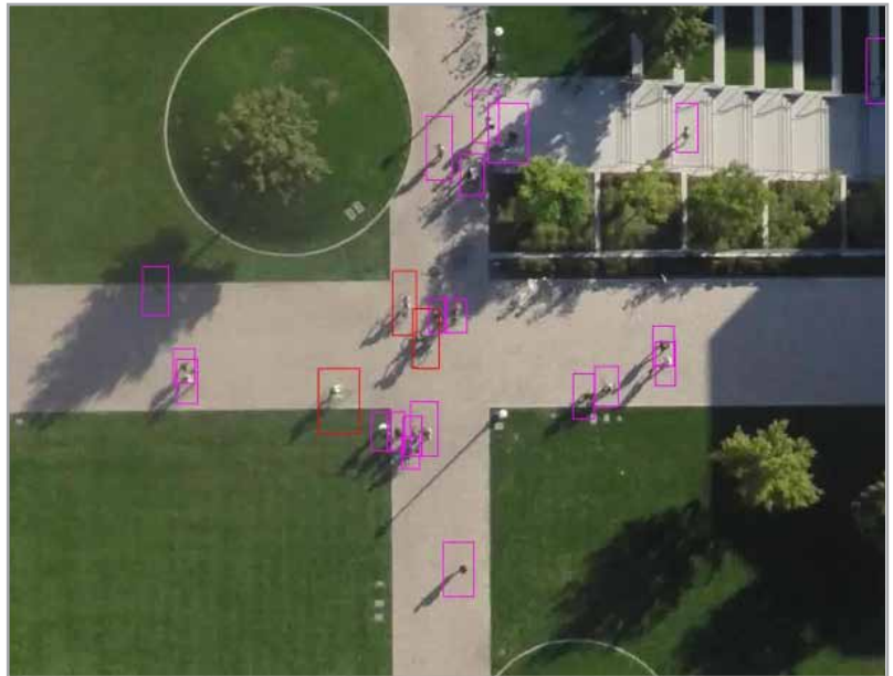
Fig. 5 - Example of pedestrian detection using YOLO on an image frame from a benchmark dataset
