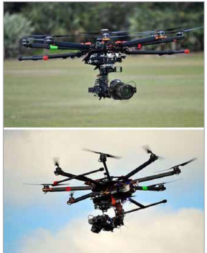
Fig. 2 - The prototype drone is an eight-copter unmanned aerial vehicle (UAV) equipped with a gimballed camera and on-board computing capabilities
