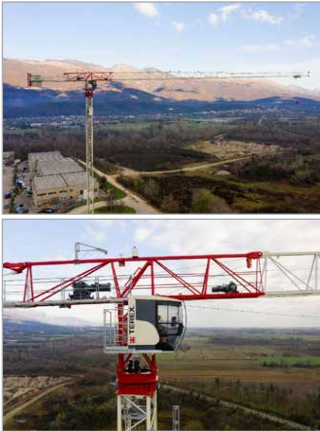
Fig. 1 - Terex flat top CTT172-8 crane
