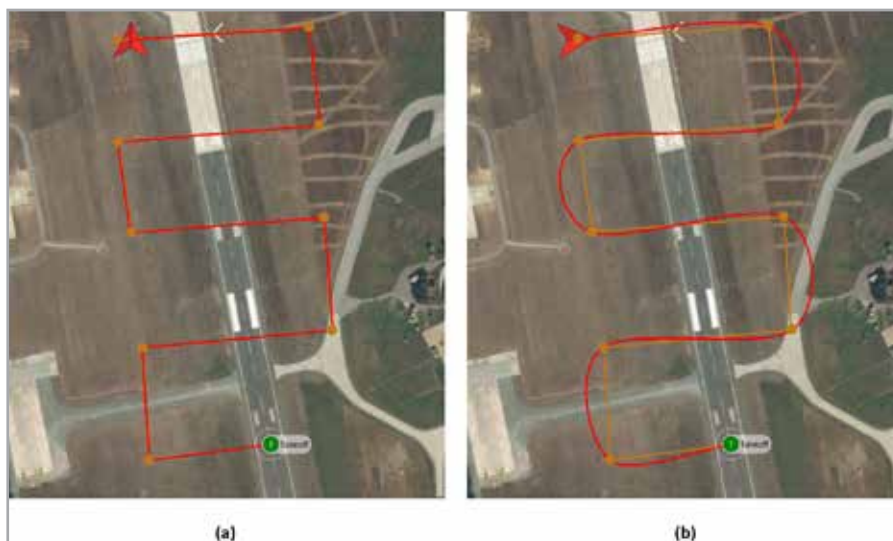
Fig. 4 - Two different trajectory models can be chosen: (a) minimum jerk trajectory, to reduce battery consumption and oscillation and (b) Hermite cubic splines to mimic the flight of a fixed-wing drone
