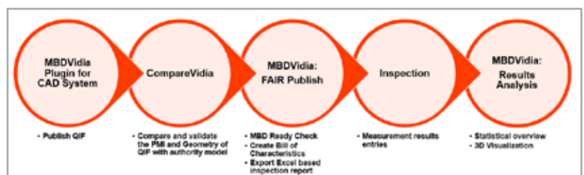
Fig. 5 – Semantic MBD-based first article inspection (FAI) form workflow
