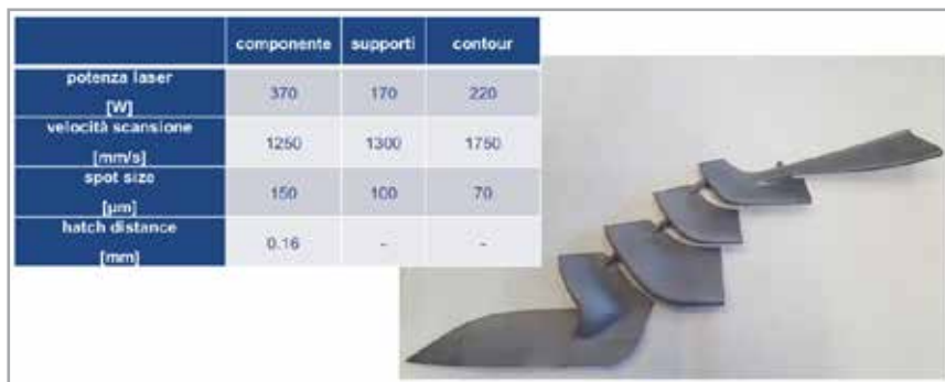
Fig. 4 – Printing parameters and final 3D printed wing (compensated geometry)
