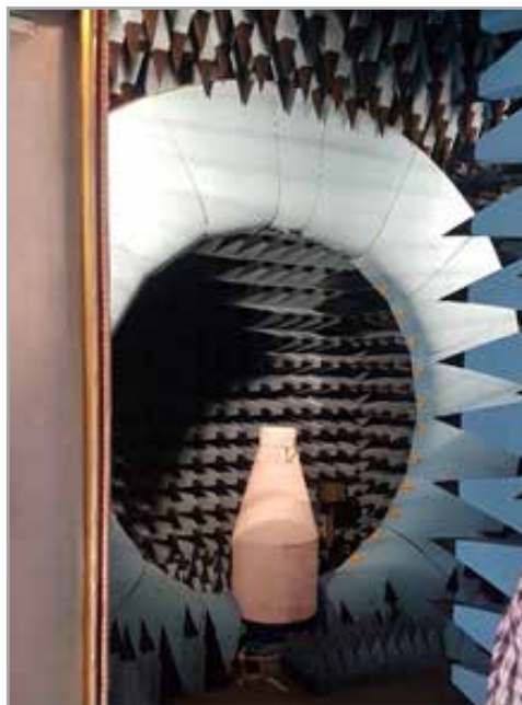
Fig. 12 – 3D radiation pattern measured in anechoic chamber
