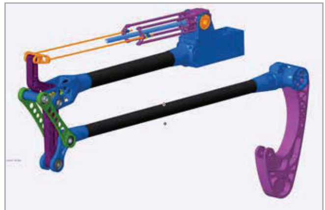
Fig. 5 - CAD design of Skippy. Real Skippy is currently being manufactured. Springs, ring screw nut and electric motor are not displayed.
