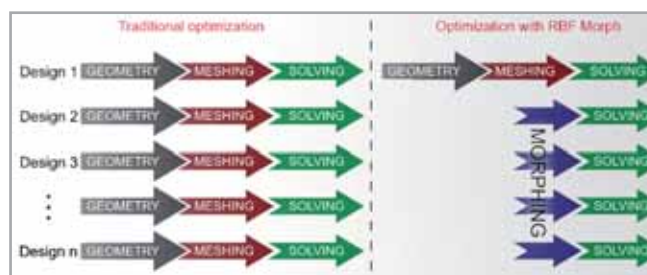
Fig. 1 - Comparison between a traditional optimization workflow and a mesh morphing-based one
