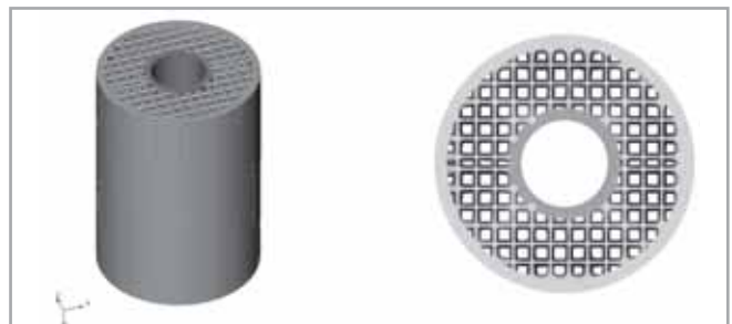
Fig. 6 - Lattice model with external skin kept
