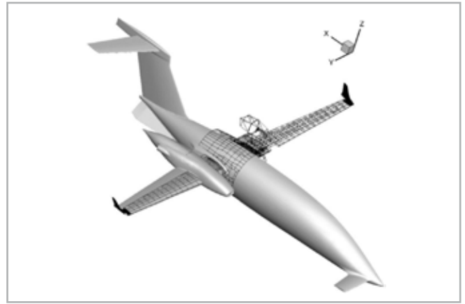
Fig. 4 - The CSM model and its position with respect to the CAD model
