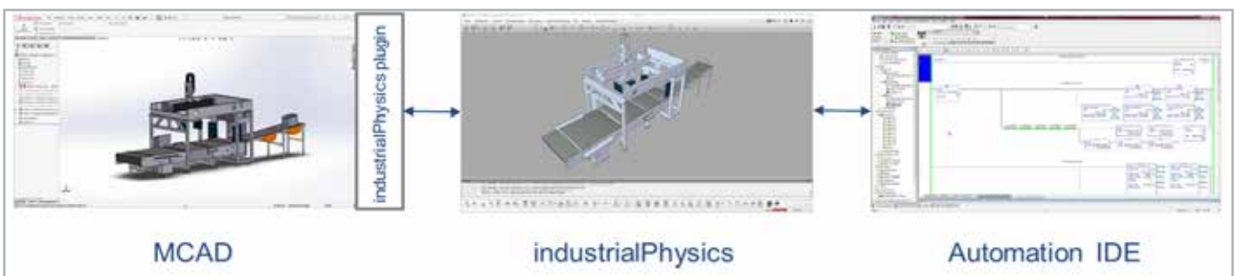
Fig. 4 - Automation developers can program in their current development IDE and test the software on the industrialPhysics simulation model
