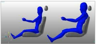
Fig. 5 - Occupant models - different anthropometrics: 5% female (left) and 95% male (right) in the RecurDvn model
