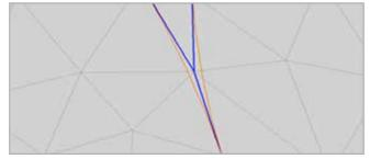
Fig. 3 - The CAD edges (orange) both use the same element edge (blue) in their edge images
