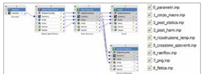
Fig. 5 - The Workbench model and the 9 macros that make up the fatigue calculation.
