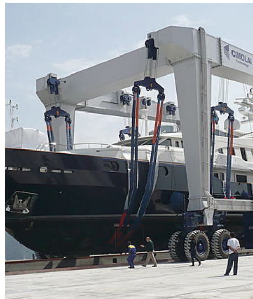
Fig. 2 - Mobile boat hauler for construction/refit yards
