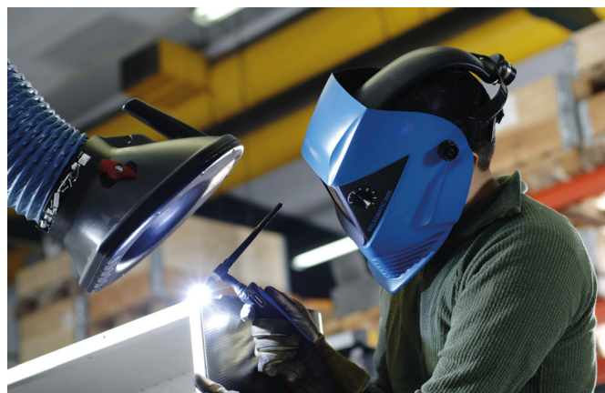
Figure 1 - Preferred welding smoke extraction: Nederman's extraction arm to extract the harmful welding fumes at the source
