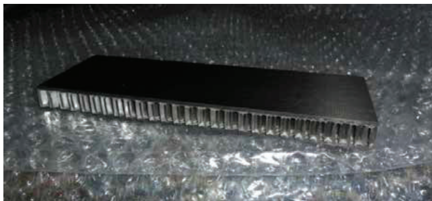
Figure 1 - Composite sandwich laminate object of the study
