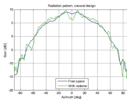
Fig. 4 - Second design, simulated radiation pattern @ 17 GHz
