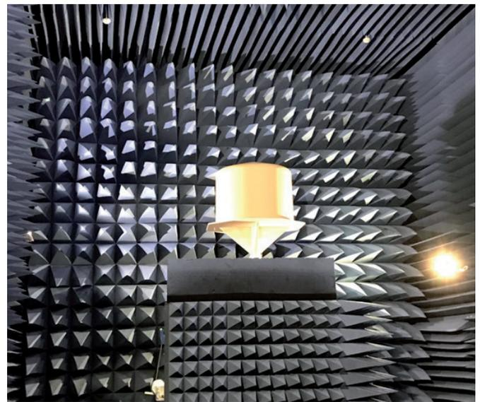
Fig. 1 - Radome in Eletttronica SpA anechoic chamber
