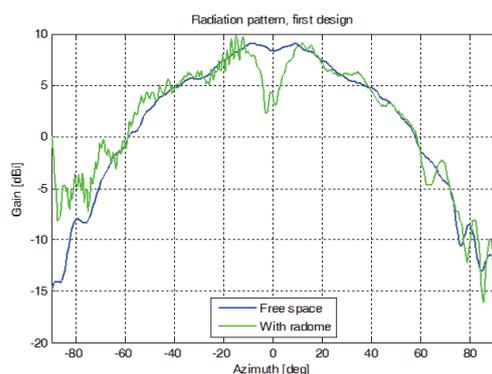
Fig. 3 - First design, simulated radiation pattern @ 17 GHz
