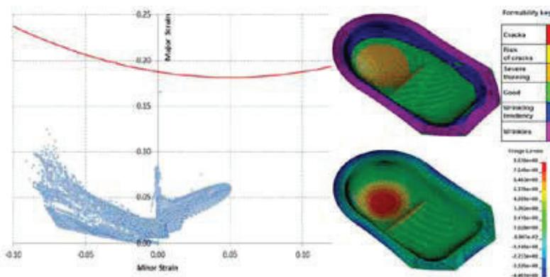
Fig. 6 - Simulation results in terms of major and minor strains of all sheet elements compared to the experimental FLC
