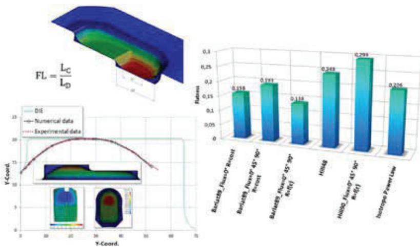
Fig. 5 - Flatness values calculated using different yield criteria
