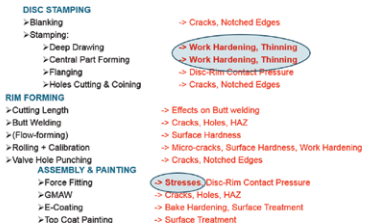
Fig. 6 - Some effects of the manufacturing process on fatigue (circled the ones analyzed in this article)
