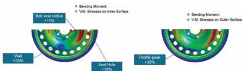
Fig. 8 - Stress distribution on the wheel after bending moment, considering the disc forming & the force-fitting processes, on inner surface (left) and outer surface (right); increments with respect to results obtained without considering the manufacturing process are indicated
