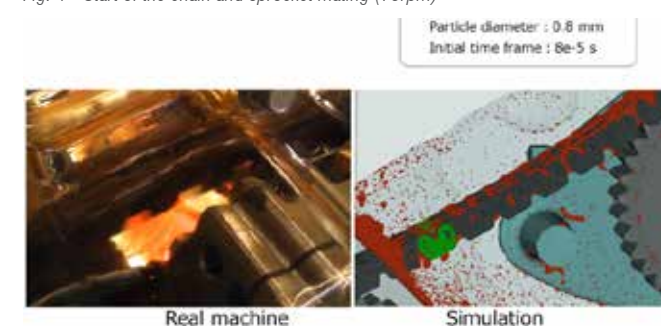
Fig. 5 – End of the chain and sprocket mating (75rpm)
