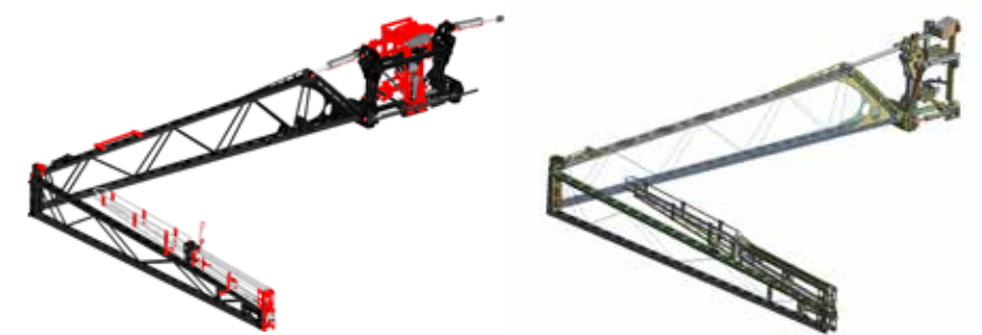
Figure 2 - On the left, original geometry for MY16 as received from CAD. On the right, geometry after the defeaturing process
