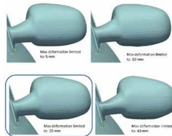
CAD Deformation According to Drag Sensitivity Map
