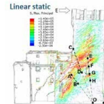
Comparison between linear static analysis results relative to a East directed force and the crack pattern suffered by the structure during the Emilia Earthquake, South front. Segments AB, CD, EF and GH correspond to the major cracks.
