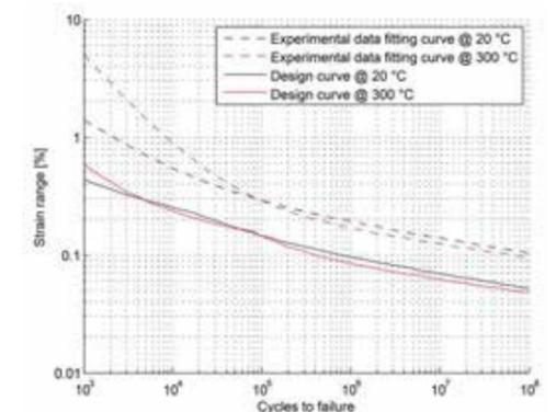
Fatigue verification of electrodeposited copper used for the grids. Strain range must be below 0.169% to perform 50000 beam on/off cycles.
