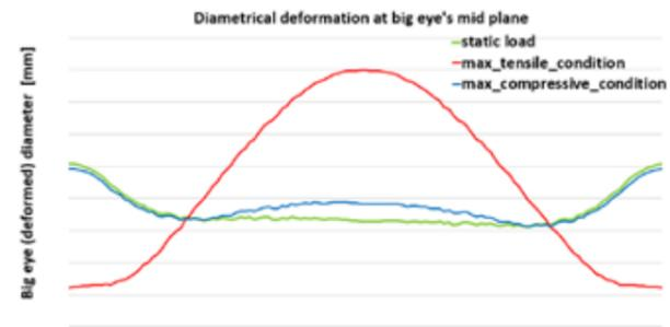
Figure 7.-Diametrical deformation of the big eye
