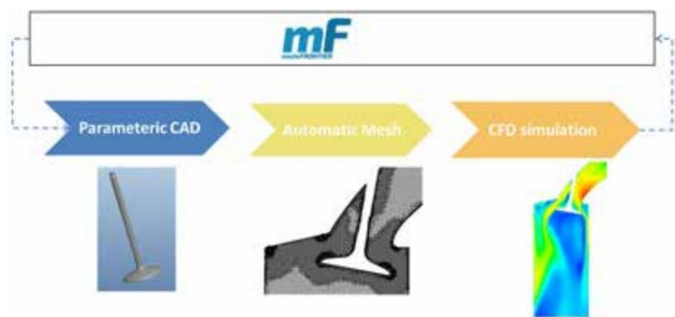
Fig.1 – Optimization process of intake valve and port
