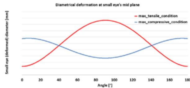
Figure 6.- Diametrical deformation of the small eye
