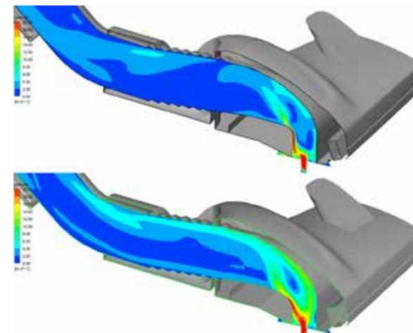
Figure 5 - New shape of the hood's elbow
