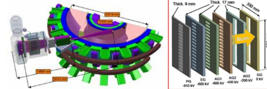
Conceptual CAD of DEMO NBI and under evaluating grids concepts (circular apertures, vertical and horizontal slots, large window)
