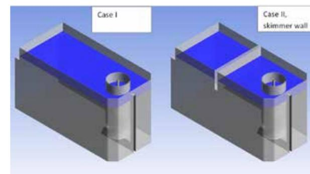
Figure 4 – Pump room CFD model: Case I (left), Case II, with skimmer wall (right)
