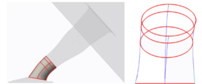
Fig.5 – Sections and splines used for the geometrical parameterization of the intake port
