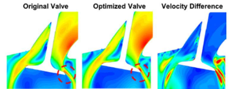
Fig.4 – Velocity field around baseline and optimized valve; velocity difference of baseline and optimized valves
