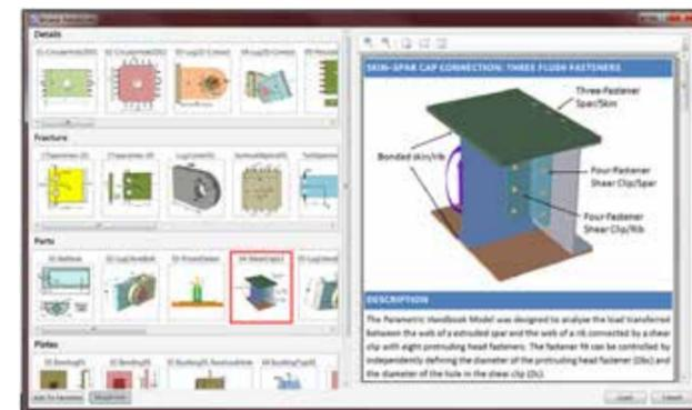
Figure 1 - Sim App example: Parametric model of an aircraft structural bolted joint
