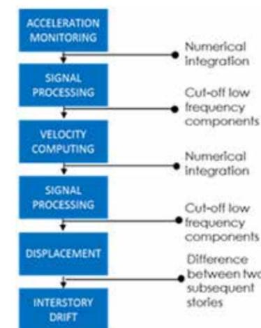
Figure 1 - Algorithm implemented in the local system for the estimation of the interstory drift
