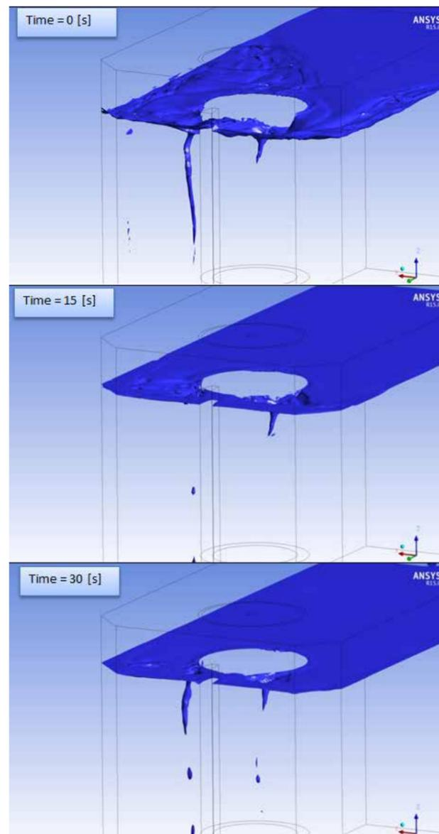
Figure 8 – Isosurface of water volume fraction at 99.5%, at time = 0[s], 15 [s] and 30 [s]
