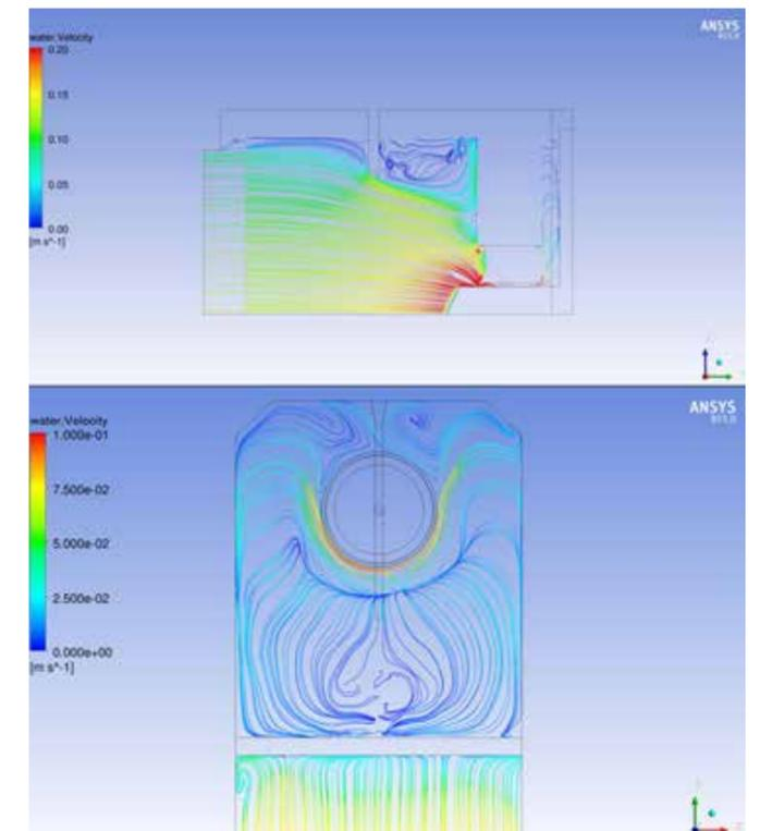
Figure 10 – Streamlines on a vertical plane and on a plane located 16.5mm beneath the free surface.
