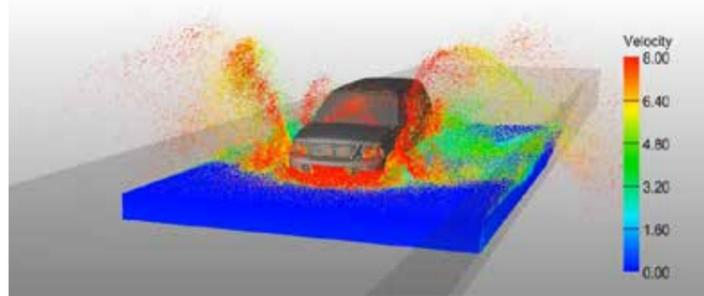
Fig.7 - Waterway driving simulation considering kinematics of vehicle and water resistance (vehicle model : FHWA/NHTSA National Crash Analysis Center)
