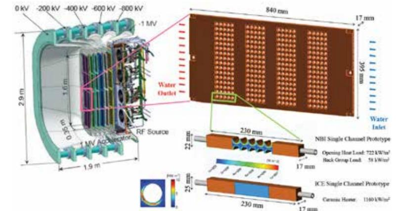
Design of the MITICA beam source. A focused view of the overall accelerating grid is shown on the left, while graphical representation of the single channel prototypes (SCP) in NBI and ICE configurations are visible below. On the bottom left a spatial estimation of the heat flux taken in input.
