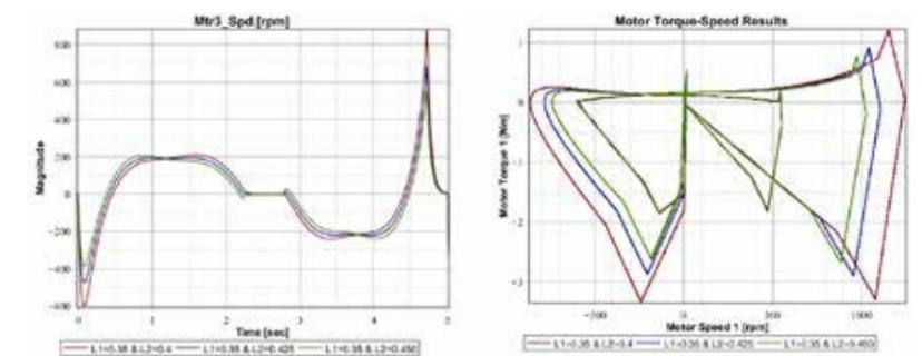
Figure 5 - Example parameter sweep results for varying link lengths
