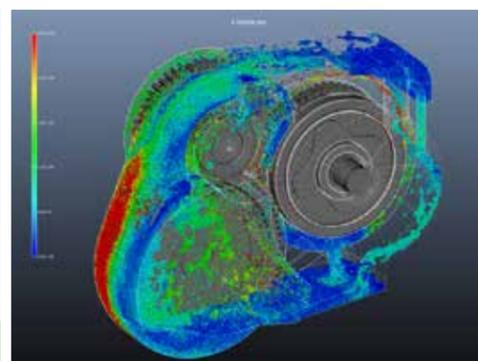
Fig.2 - Example of simulation using Particleworks: Oil lubrication in a gear box
