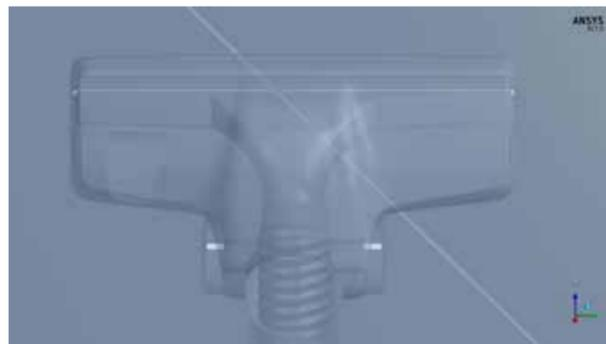
Figure 2 - CFD model of the Vacuum Cleaner
