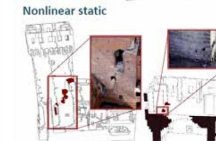
Nonlinear static analysis for a horizontal East directed force, North front. The computed damaged zones are highlighted in red.
