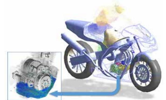
Fig.5 - Simulation of lubrication oil behavior in an engine of motorcycle from start-up to traveling (Courtesy of Thomas Freviller and FunctionBayK.K.)
