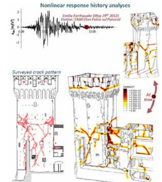
Constitutive model: Concrete Damage Plasticity (Lee, J. et al, 1998). Analysis type: Dynamic Explicit (Abaqus© 6.11). Plots refer to the tensile damage variable (DAMAGET).
