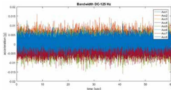
Figure 5 - Accelerations recorded during the earthquake of Rieti 24/08/2016
