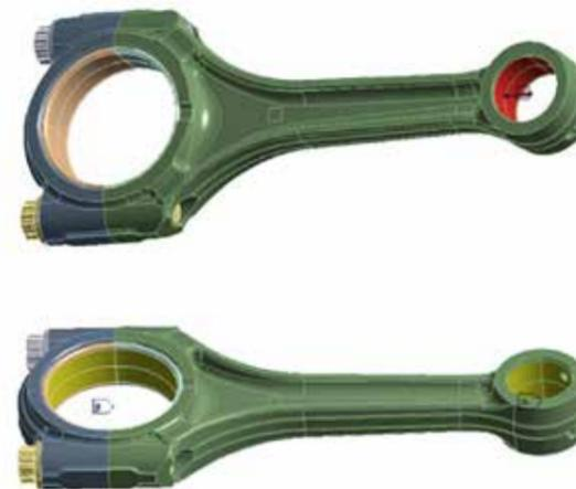
Figure 3 - Boundary conditions for the buckling analysis
