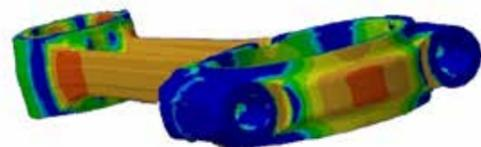
Figure 9 - Safety factor distribution with quasi-static superposition analysis
