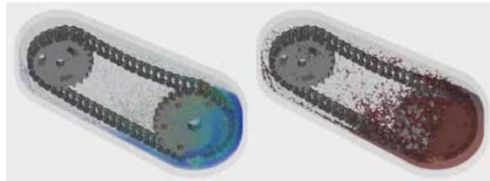
Fig.6 - Lubricant behavior inside the housing of a transmission chain mechanism (Model geometry: courtesy of Amine, member of mechatronics INSAT)
