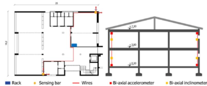
Figure 4 - Scheme of the monitoring system
