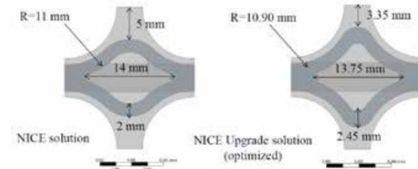
Schematic representation of NICE design pre and post optimization (left), bubble chart showing the pareto region in a  $T_{max} - \Delta p$  plot (right).
