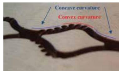
SCP copper slab (right) and detailed view of the inclined ribs in Tilt Turbotron concept (left)
