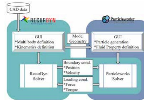
Fig.3 - Schematic flow of MBD-fluid co-simulation using RecurDyn and Particleworks
