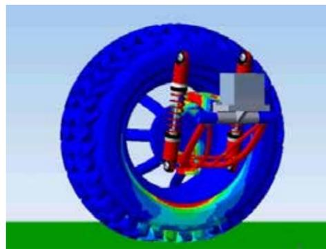
Fig.1 - Example of simulation using RecurDyn: Buggy car suspension system behavior including tire deformation
