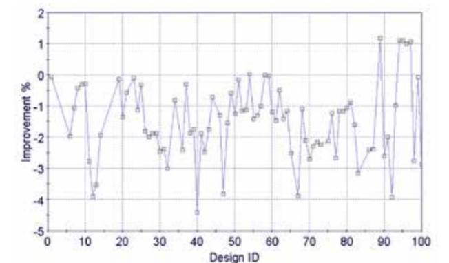
Fig.6 – Optimization results with modeFRONTIER: % improvement of intake overall mass flow rate
