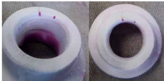
Fig. 2 - Example of cracks on a finished part
