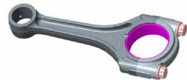
Figure 1 - 3D geometry of the connecting rod
