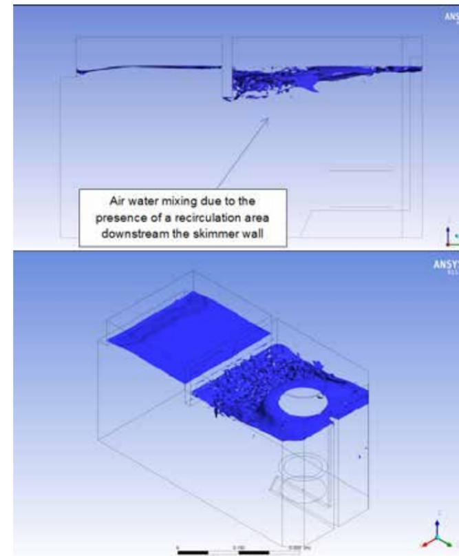
Figure 9 – Isosurface of water volume fraction at 99.5%
