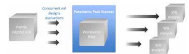
Figure 1 - Usage of ANSYS HPC Parametric Pack in modeFRONTIER optimization software
