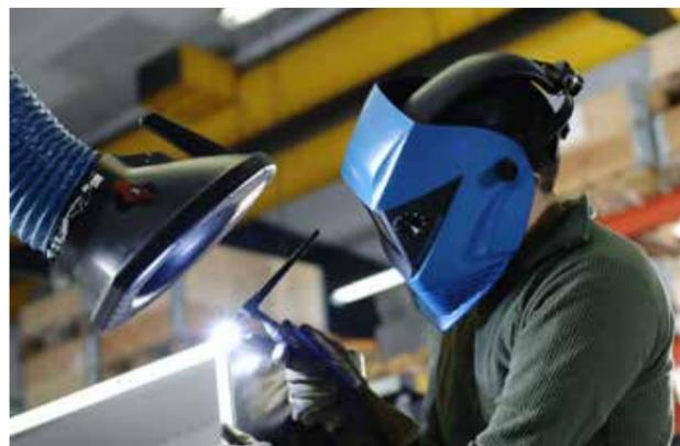
Figure 1 - Preferred welding smoke extraction: Nederman's extraction arm to extract the harmful welding fumes at the source
