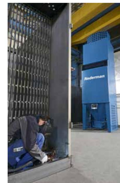
Figure 5- Nederman's new Air Purification Tower
