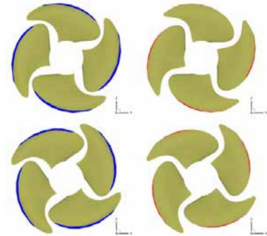
Fig. 6 - Comparison of predicted unsteady face cavity extension (0° - 60°) between original (left, blue) and optimized (right, red) propeller at reduced pitch [Bertetta et al 2012]
