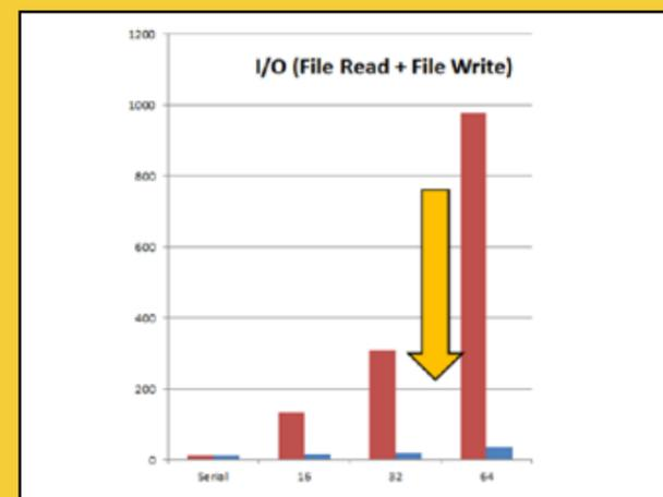
Figure 1: Reduction in wall clock seconds for I/O on an example test case with many regions
