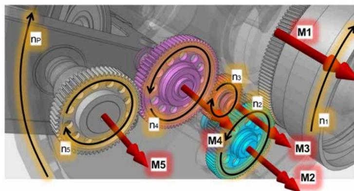
Figure 4 – Planetary gear unit
