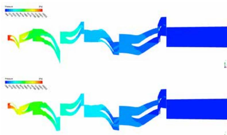
Figure 15 - Three stage, single passage - CFD model with actual sealings and cavities - Static pressure field comparison @ 50% span - Baseline (above) and optimized (below)
