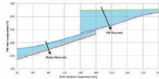
Fig. 3 - Maximum temperature of the thermocouple T30 at 20<sup>th</sup> cycle versus fluid medium temperature, flow rate from 0.2 m<sup>3</sup>/h to 2.4 m<sup>3</sup>/h
