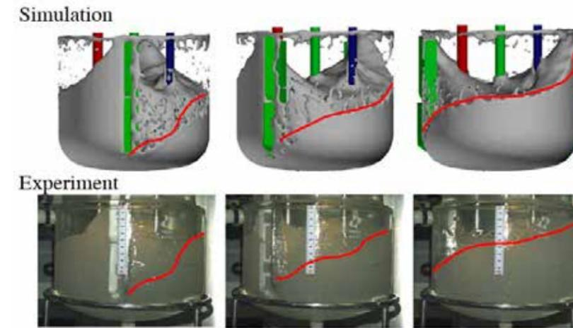
Fig.2 - Comparison of mixing states of 3.5 liters of fluid A with an anchor rotation of 90 rpm. The red line shows the depth of free surface at the rear side of the anchor
