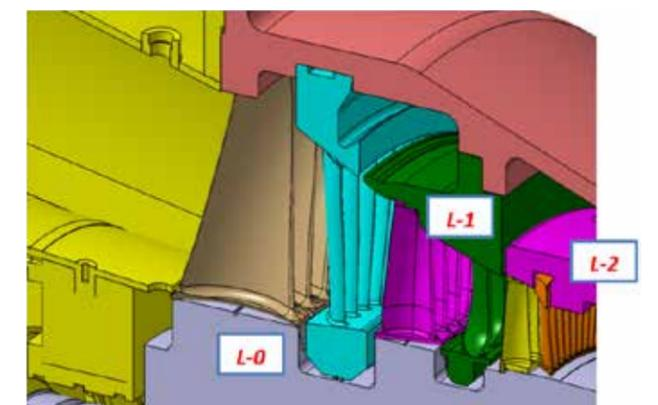
Figure 2 – Multi-stage steam turbine design by Franco Tosi Meccanica – Details of the last three low-pressure stages – Sealings and cavities
