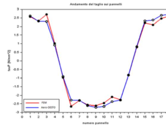
Figure 11 - FEM vs AeroDESTO tool solution
