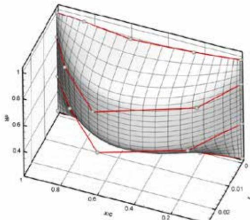
Fig. 2 - Parametric representation of propeller nondimensional mean surface [Bertetta et al 2012]
