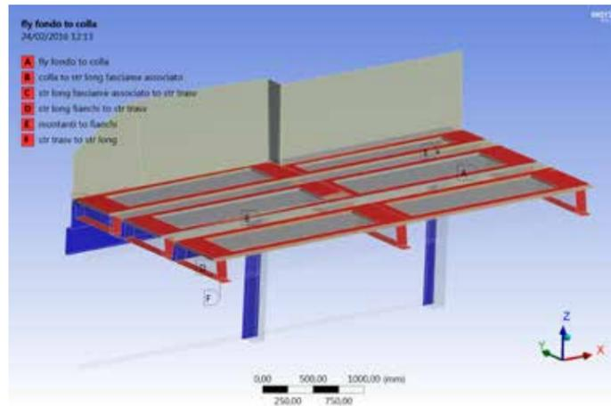
Figure 3 - Mechanical allows to insert connections among parts defining how parts interact with each other
