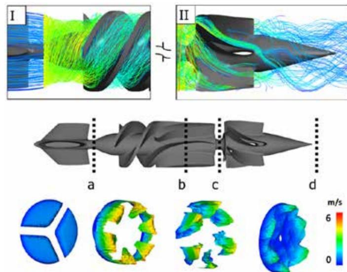
Fig. 4 – Upper panels: streamlines calculation to highlight the velocity field before (I) and after (II) the rotor. Lower panels: velocity magnitude (m/s) 3D contours on different cross-sectional planes (a – d)
