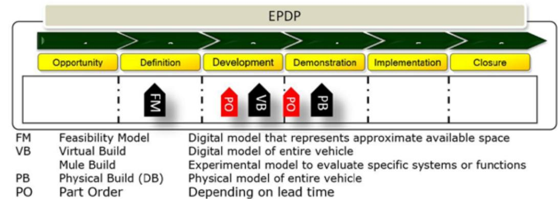
Figure 2 – The way to use simulation and experiment in the right sequence
