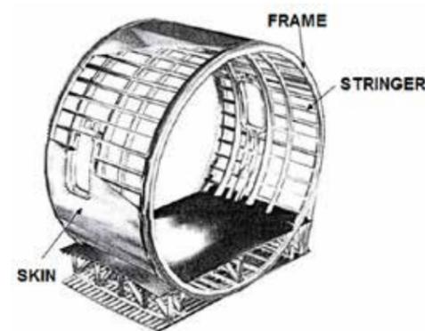
Figure 1 - Typical fuselage section
