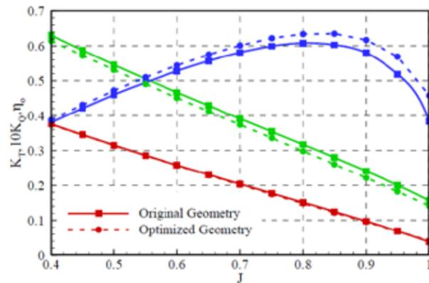
Fig. 7 - Comparison between original and optimized propeller – open water tests – reference pitch [Bertetta, D., Savio, L. and Viviani, M. 2011. Experimental characterization of two CP propellers at different pitch settings, considering cavitating behaviour and related noise phenomena, SMP 2011]
