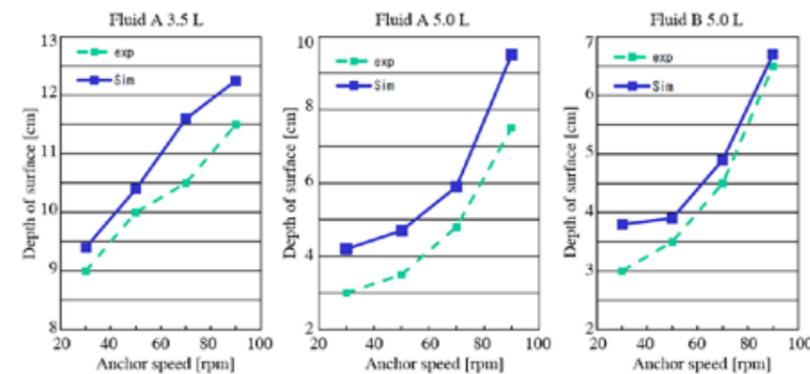
Fig.3 - Depth of surface at rear side of anchor
