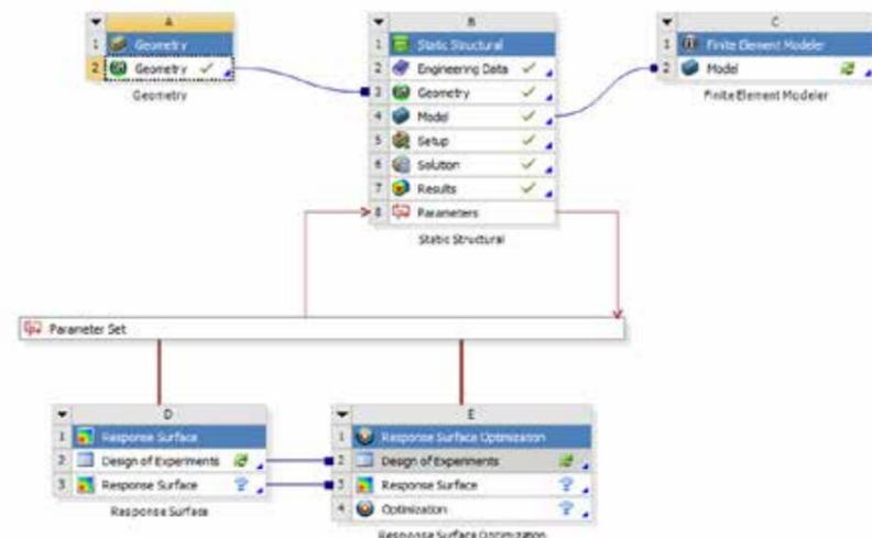
Figure 4 - Optimisation workflow in ANSYS Workbench. A geometrical model is used to generate the baseline (a static analysis in this example). Input parameters (that feed RBF Morph) and output parameters (computed by FEM solver) are steered by the optimization software DX (adopting in this case a response surface method). Optimal design point is sent to FEModeler that allows to generate the CAD of the new shape
