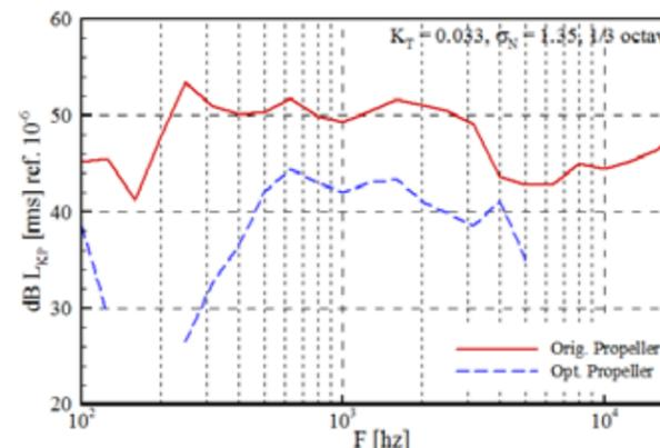
Fig. 12 - Radiated noise measurements at reduced pitch [Bertetta et al 2012]
