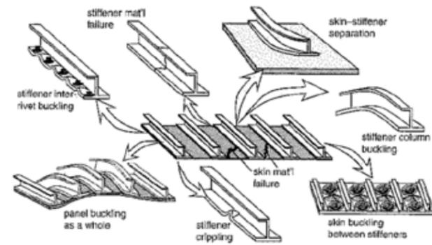
Figure 6 - Failure mode of aeronautical panel and stringer
