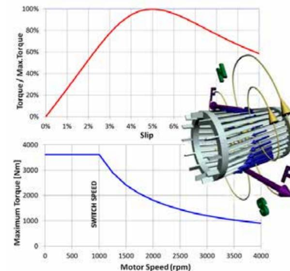
Figure 5 – Induction motor model
