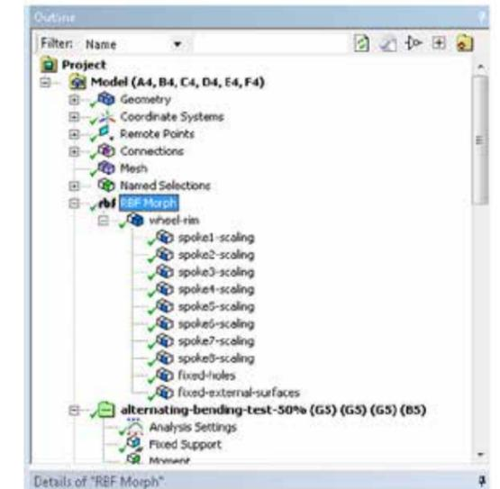
Figure 6 - A detail of the Tree in Mechanical; RBF Module acts just before the mesh generation and the definition of the Named Selections. It's comprised of a set of target nodes (wheel-rim), of 8 set of source nodes controlled by a scaling (spoke1-scaling, spoke2-scaling,...,spoke8-scaling) and of two set of fixed nodes (fixed-holes, fixed-external-surfaces)
