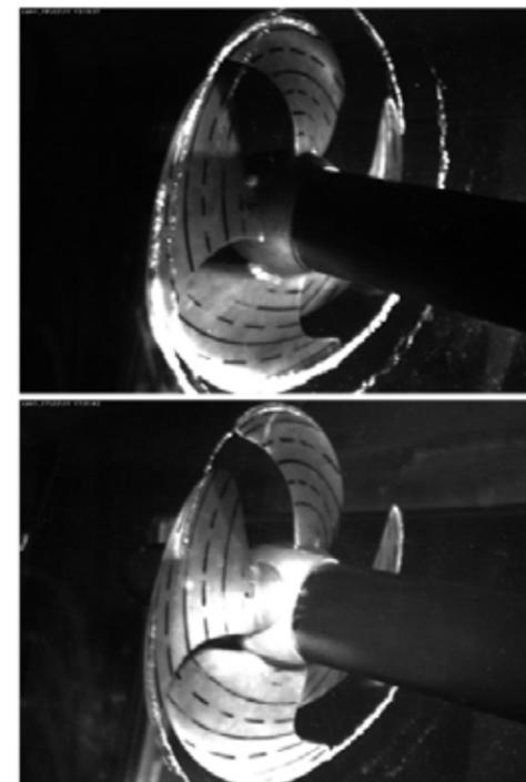
Fig. 10 - Observed cavitation extent at reduced pitch Original propeller (above) vs optimized propeller (below) [Bertetta et al 2012]
