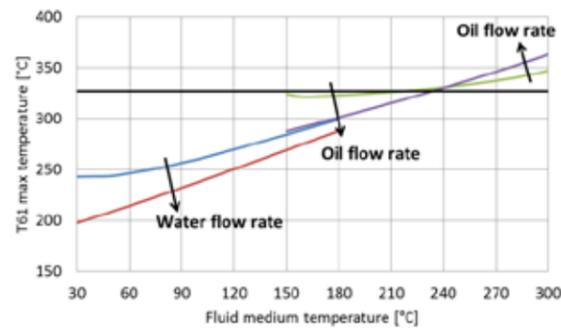
Fig. 9 - Maximum temperature of thermocouple T61 versus fluid medium temperature, flow rates from 0.2 m³/h to 2.4 m³/h
