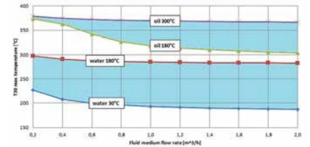
Fig. 4 - Maximum temperature of the thermocouple T30 at 20<sup>th</sup> cycle versus fluid medium flow rate
