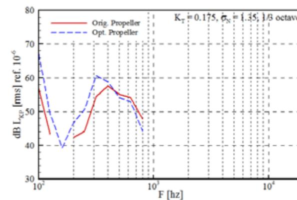
Fig. 11 - Radiated noise measurements at reference pitch [Bertetta et al 2012]
