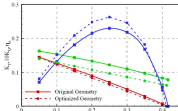
Fig. 8 - Comparison between original and optimized propeller – open water tests – reduced pitch [Bertetta et al 2012]
