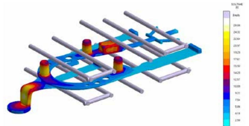
Fig. 5 - Solidification time at 15th cycle
