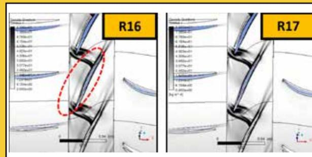
Figure 5: Enhancements to Stage (Mixing-Plane) model allow to avoid spurious results across interface
