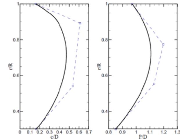
Fig. 1 - B-Spline representation of radial distributions of chord and pitch. [Bertetta, D., Brizzolara, S., Gaggero, S., Viviani, M., Savio, L. 2012 "CP propeller cavitation and noise optimization at different pitches with panel code and validation by cavitation tunnel measurements", Ocean Engineering 53 (2012)]
