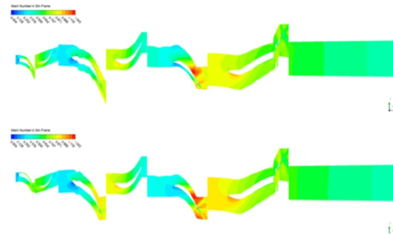
Figure 16 - Three stage, single passage - CFD model with actual sealings and cavities - Mach number field comparison @ 50% span - Baseline (above) and optimized (below)
