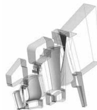
Figure 13 – Three stage, single passage – CFD model with actual sealings and cavities
