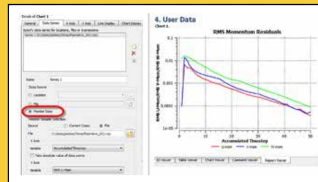
Figure 6: CFX Monitor Data are available directly in CFD-Post
