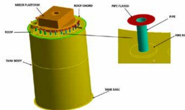
Figure 1 - 3D geometry and parts of HX62-CM002 tank
