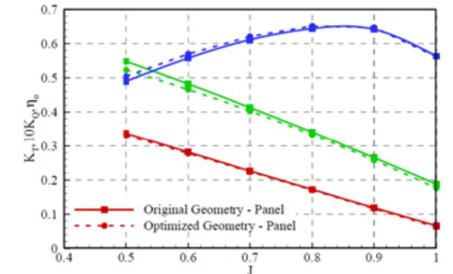
Fig. 4 - Comparison between original and optimized propeller - numerical open water tests - reference pitch [Bertetta et al 2012]
