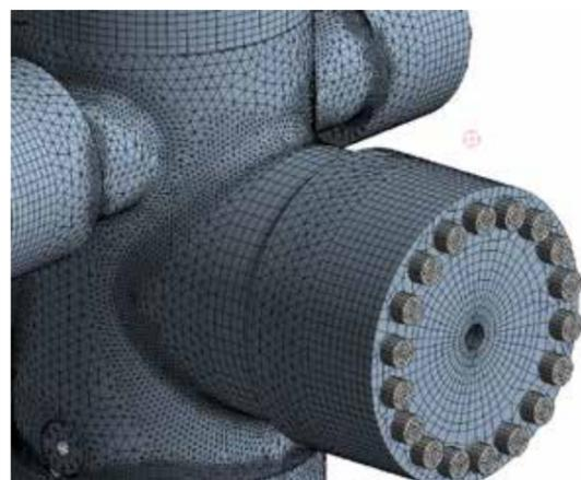
Figure 3 - Finite Element Model of a Well Head Safety Valve - Detail
