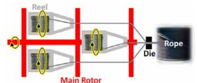
Figure 1 – Planetary stranding machine scheme
