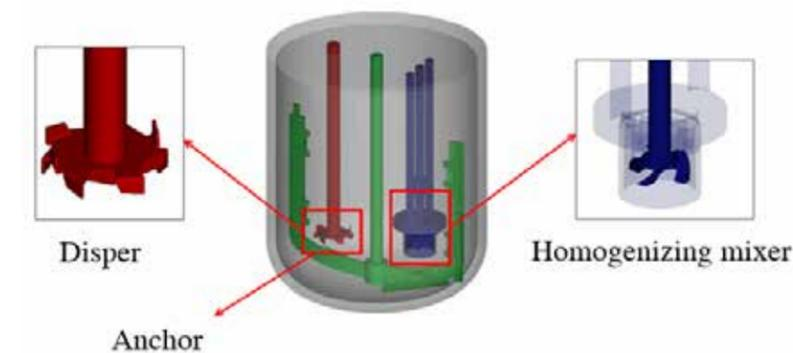
Fig.1 - Example of the mixing system for emulsification and dispersion
