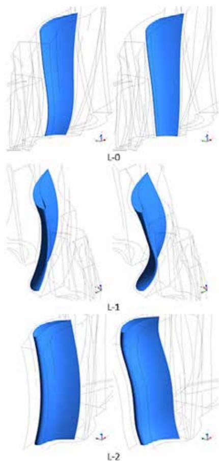
Figure 11 – Comparison between baseline (left) and optimized (right) design of the statoric blades – Blade geometry
