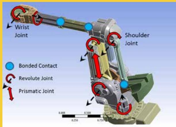
Figure 2 - Rigid Body Dynamics using rigid and flexible bodies
