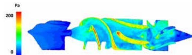
Fig. 5 – Wall shear stress computation (Pa) to highlight high-risk locations of the device prone to blood damage
