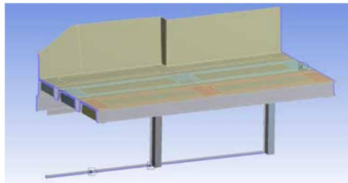
Figure 4 - Bases of struts are fixed by displacement bounds; the aft, the fore and the bottom contour are simulated by fixed supports on their edges
