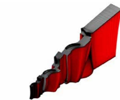
Figure 5 – Three stage, single passage – Computational grid
