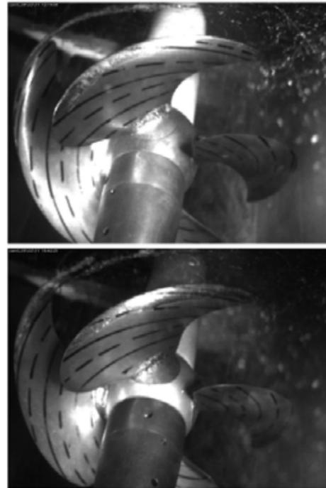
Fig. 9 - Observed cavitation extent at reference pitch Original propeller (above) vs optimized propeller (below) [Bertetta et al 2012]
