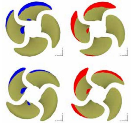
Fig. 5 - Comparison of predicted unsteady back cavity extension (0° - 60°) between original (left, blue) and optimized (right, red) propeller at reference pitch [Bertetta et al 2012]
