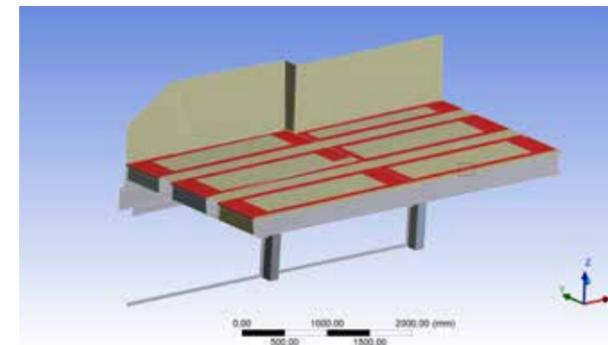
Figure 2 - Closed volume, representing the glue volume of 15 mm thickness
