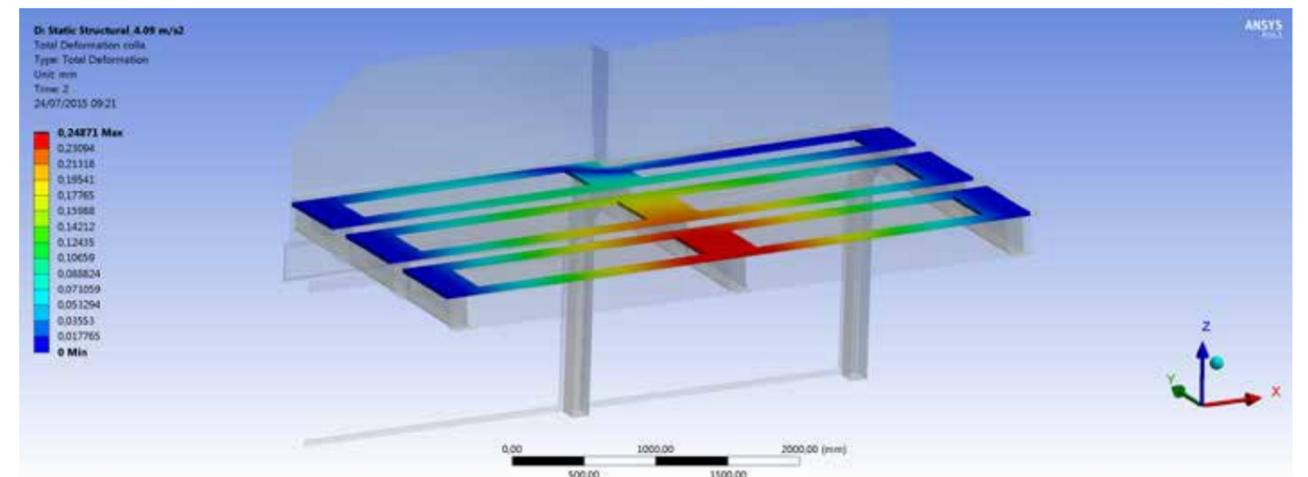
Figure 5 - Only 0.2 mm deformation at the centre zone of the 15 mm glue inserted to join the fly to the deckhouse structures
