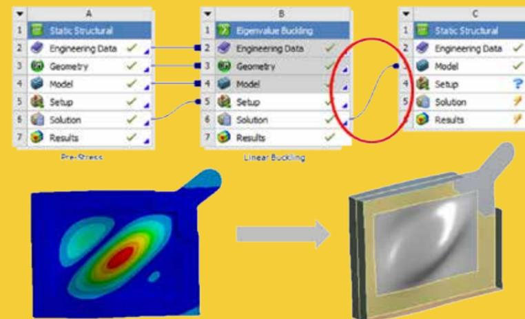
Figure 6 - Automatic export of deformed mesh and geometry using links in ANSYS WB
