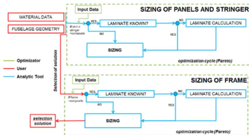
Figure 4 - Tool logic flow chart
