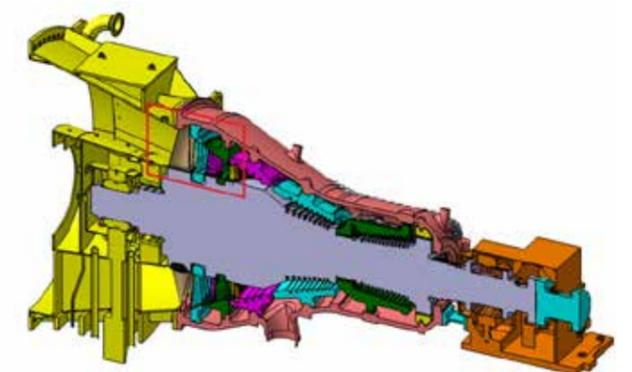
Figure 1 – Multi-stage steam turbine design by Franco Tosi Meccanica – The last three low-pressure stages are highlighted in the red box
