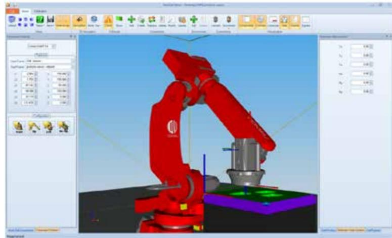
Figure 2 - Workcell Simulator used to set a quality control cycle in a cell with viewing system mounted on a robot
