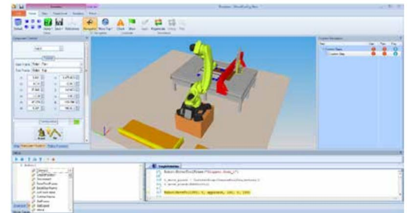
Figure 1 - Workcell Simulator used to program a wood cutting cell with a robot
