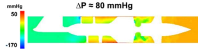
Fig. 3 – Static pressure (mmHg) contour on a longitudinal plane to highlight the pressure head of the device
