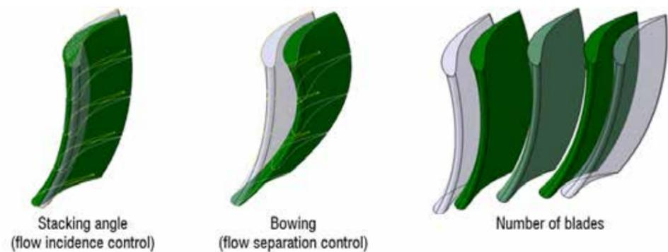
Figure 3 – Blade geometry – Description of parameters
