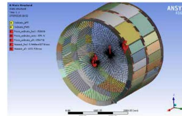
Figure 10 - FEM model of fuselage section
