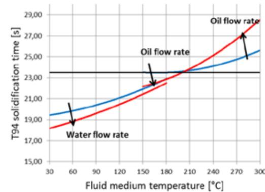
Fig. 7 - Solidification time of the casting versus fluid medium temperature (blue lines mean 0.2 m³/h, red lines mean 2.4 m³/h, black line means no cooling channels)
