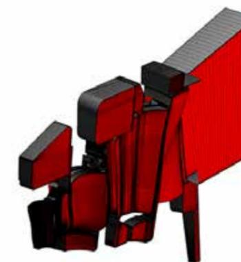
Figure 14 – Three stage, single passage – Computational grid with actual sealings and cavities
