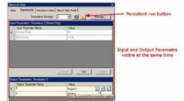
Figure 1 - Persistent run button and visualisation of input and output parameters
