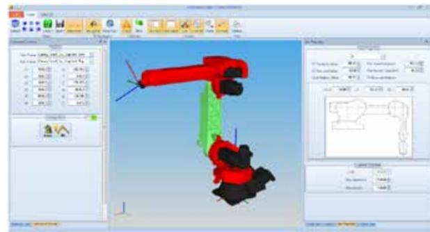
Figure 3 - Six-axis robot editor. It allows static and dynamic robot features to be customised
