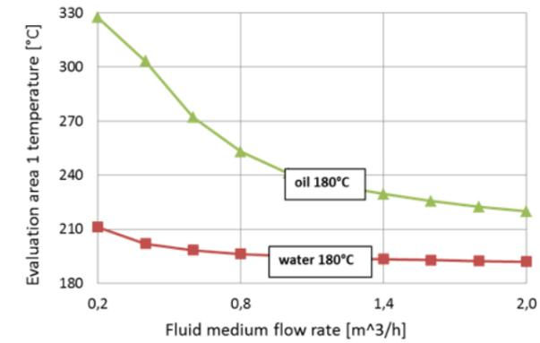
Fig. 2 - Temperature of Evaluation Area 1 at 20<sup>th</sup> cycle versus fluid medium flow rate
