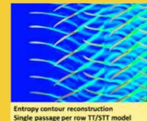
Figure 3: Transient Blade Row – Multi-stage Time Transformation method
