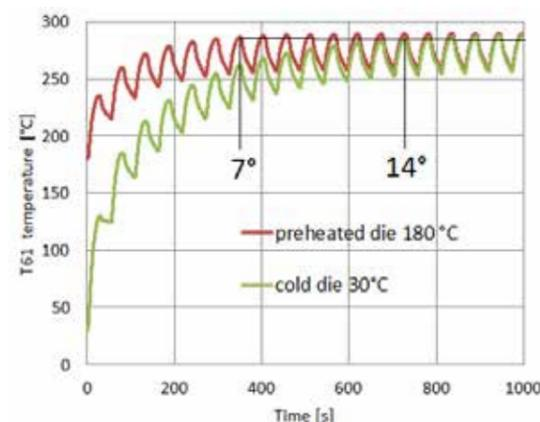
Fig. 10 - Temperature distribution during the dies heating
