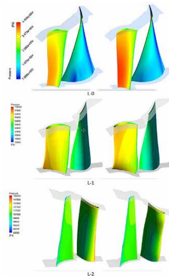
Figure 12 – Comparison between baseline (left) and optimized (right) design of the statoric blades – Pressure field on blades
