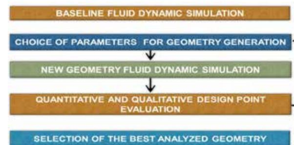
Figure 7 – Optimization methods – “Trial-and-error” approach
