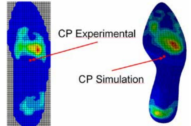
Fig. 5 – Comparison between experimental plantar pressure (left) and numerical plantar pressure (right) for shoe nr. 2 and CP – Centre of Pressure
