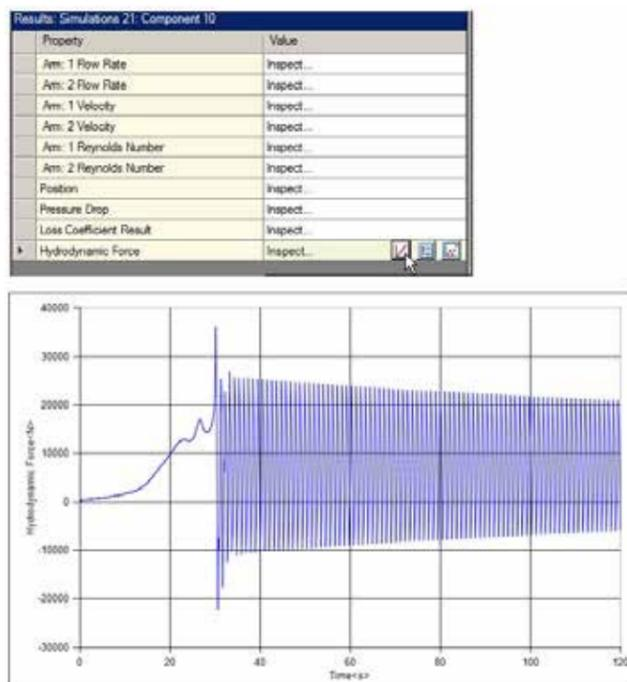
Figure 5 - Hydrodynamic force on a pipe during a water hammer
