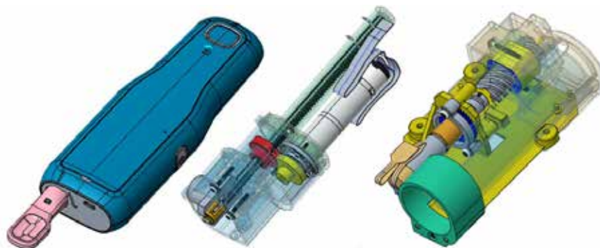
Fig. 2. Technology demonstrator of an autoinjector - CAD model.
