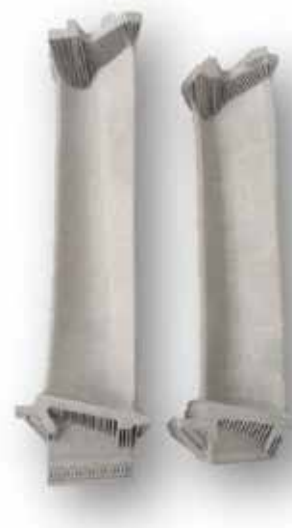
Fig.1. Example of EBM LPT blades before any HT.
