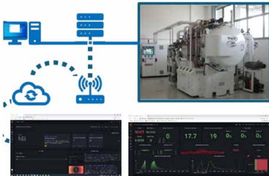
Fig.2. Diagram of the digital platform and its integration into the production line.
