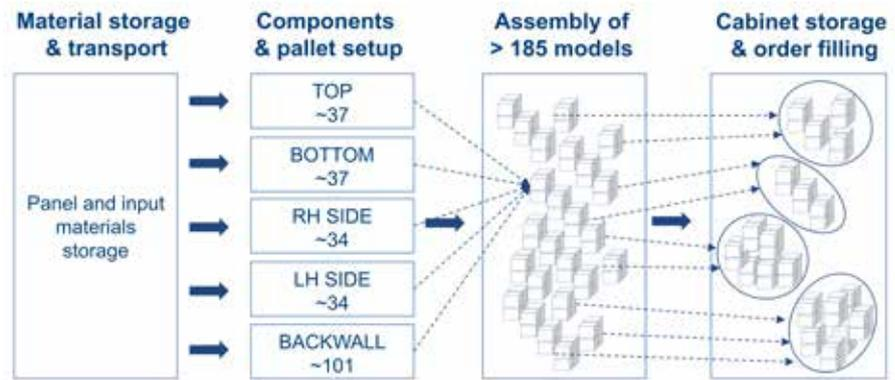
Fig.3. Diagram of material flow and data collected for simulation.
