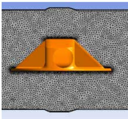
Fig. 3. CFD model for open disc pressure drop analysis.
