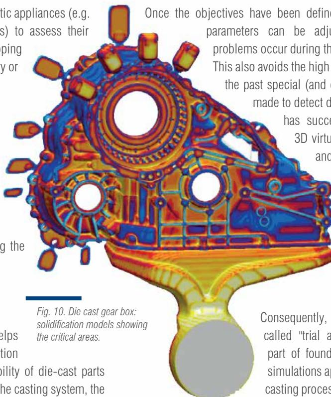
Fig. 10. Die cast gear box: solidification models showing the critical areas.
