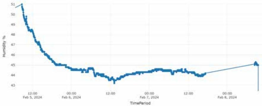
Fig.1. Time series analysis of humidity values during the injection moulding process.
