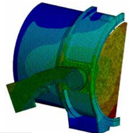
Fig. 6. Displacement range for valve in closed position.
