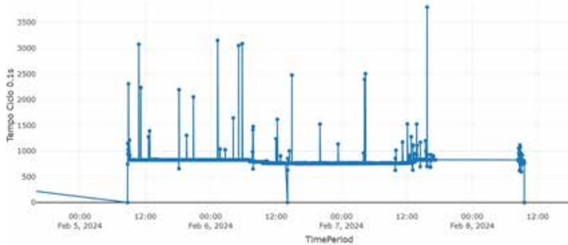
Fig.3. Cycle time (Tempo Ciclo) [0.1s] of the injection moulding process from 5–8 February 2024.
