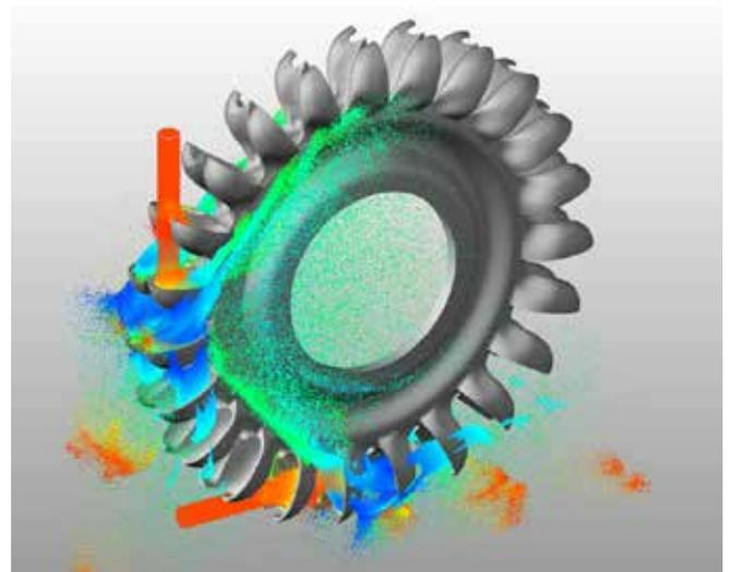
Fig. 15. Application of MPS to optimize power generation from Pelton turbines.
