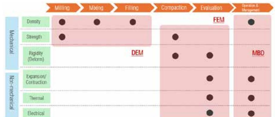
Fig.3. Material constants governing each step in the dry production process of all-solid-state batteries.
