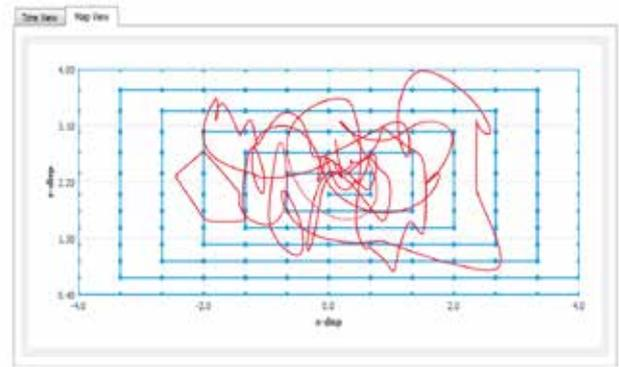
Fig.3. Two-channel map discretizing a space defined by the  $x$  and  $z$  displacements. Blue dots represent FE solutions for which the stress-strain fields are precomputed. The blue line represents a solution path, which defines the order in which the solutions are computed and stored in the results database. The red line represents a possible actual displacement history. The stress-strain history for points on the red path is obtained by interpolation from points on the precomputed map.
