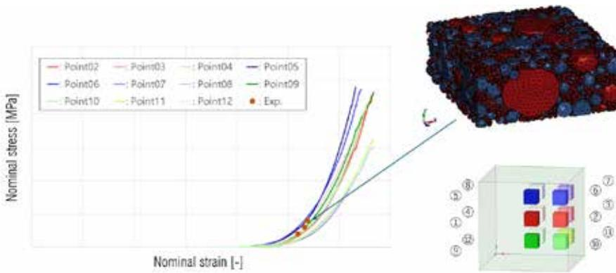
Fig.6. Stress-strain curves at 12 typical locations, obtained by compression analysis. The analysis results could be validated in the small strain region. (Specific value for each axis is hidden for confidentiality).
