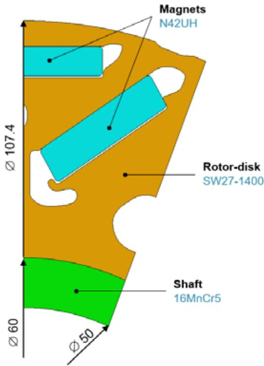
Fig. 4. Rotor plate of an electric motor.
