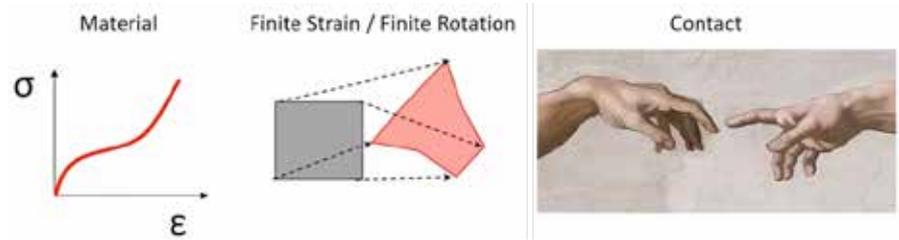
Fig.1. Nonlinearity figures in the analysis of rubbery materials in several ways including material nonlinearity, kinematic nonlinearity, and contact linearity. Endurica's EIE solver provides an efficient and accurate method for generating stress-strain history when there is strong nonlinearity.
