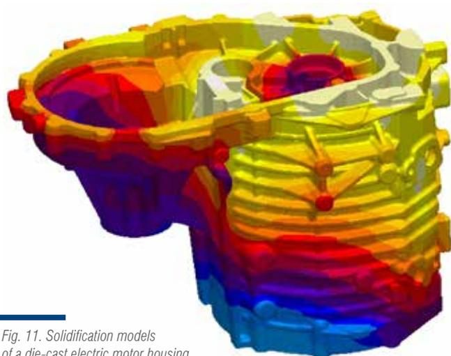
Fig. 11. Solidification models of a die-cast electric motor housing.
