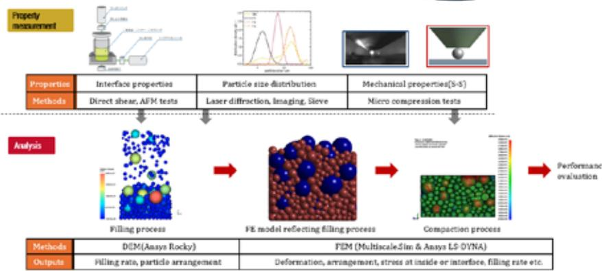
Fig.4. Workflow to simulate a series of manufacturing processes using DEM-FEM coupling.
