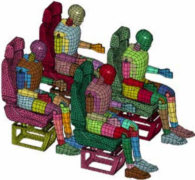
Fig. 8. Hybrid III 50th percentile male LSTC virtual dummies positioned in the cabin of a special vehicle.
