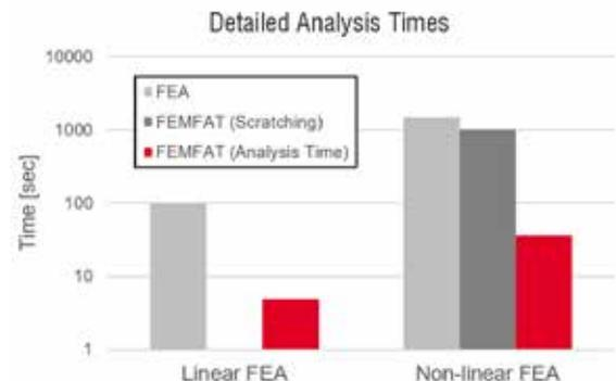
Fig.6. Analysis time for finite element analysis (FEA) and fatigue analysis.
