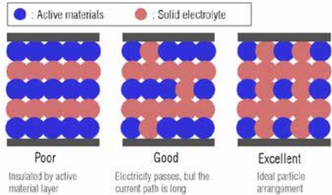
Fig.2. The relationship between microstructure and performance of all-solid-state batteries
