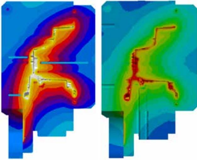
Fig. 13. a) Temperature distribution at cavity transferred from casting simulation to b) Structural simulation to assess the thermal steady state stress analysis.
