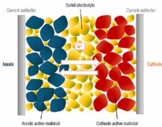
Fig.1. Diagram of the internal microstructure of an all-solid-state battery.
