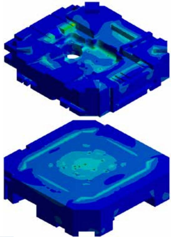
Fig. 14. Von Mises stress distribution in some structural components of the die casting tool.
