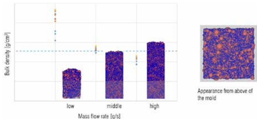
Fig.5. Analysis of the filling step of the process as a function of particle mass flow rate.
