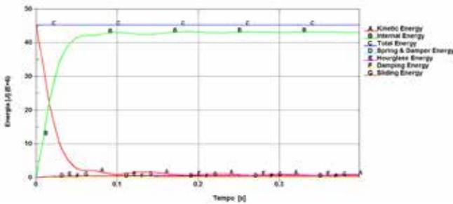
Fig. 9. Energy balance of a frontal impact on the cabin of a special vehicle.
