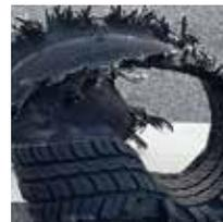
36 Rubber fatigue ≠ metal fatigue: mean strain effects
