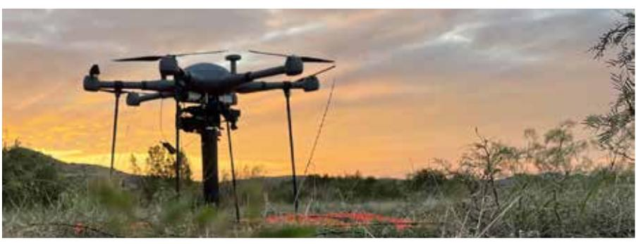
As part of the development exploration into the application of the True-Load technology, Menet agreed to swap out the carbon-fibre arms with thin aluminium tubes. This would allow for easier FEA modelling and simpler strain gauge application. The plan is to follow up with a carbon-fibre FEA model and specialized carbon-fibre strain gauges once the demonstration has been successfully completed.
