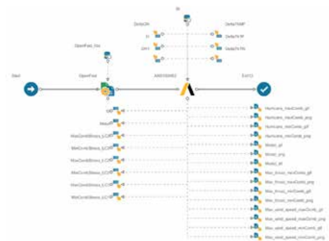
Fig. 2. Automated workflow in modeFRONTIER to minimize the mass of the offshore wind turbine monopile.
