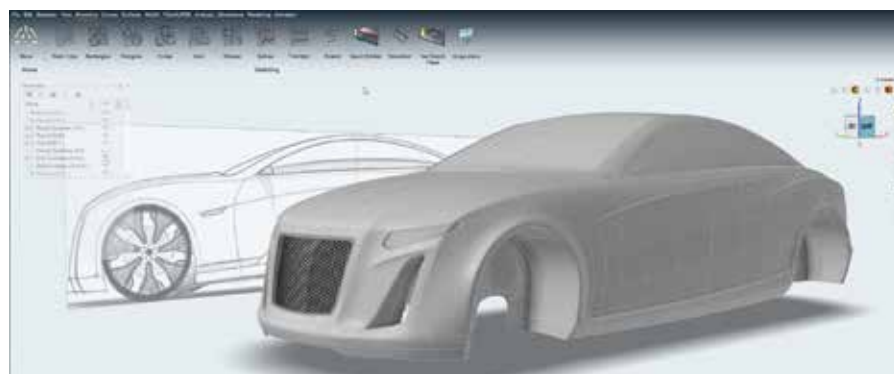
When sub-division surface modeling software is tailored for CAE a detailed open grille vehicle model can go from an idea on paper to a fully detailed simulation mesh in one business day.
