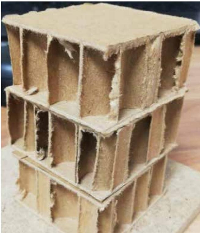
Fig. 1 - Paper honeycomb samples.
