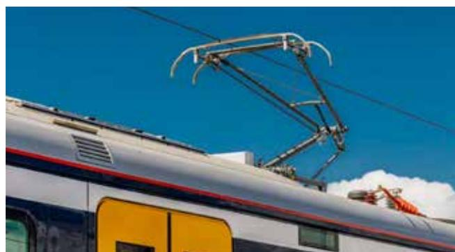
Fig. 1 - The pantograph of a high-speed train.
