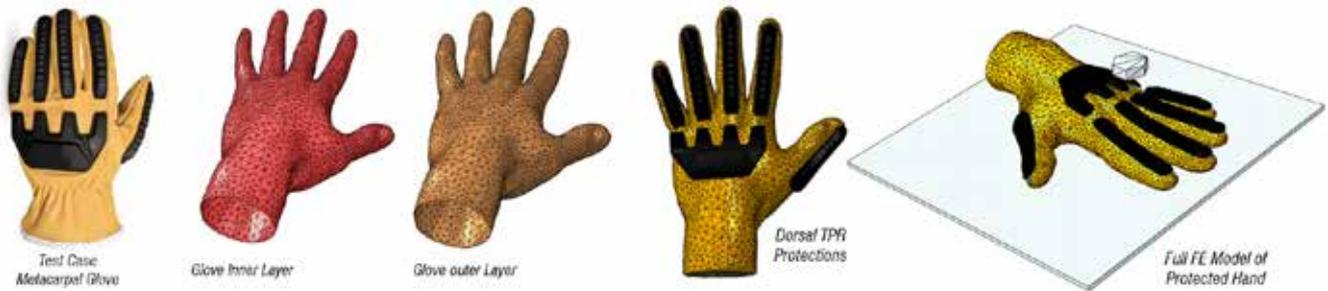
Fig. 3 - Finite element model of metacarpal glove.
