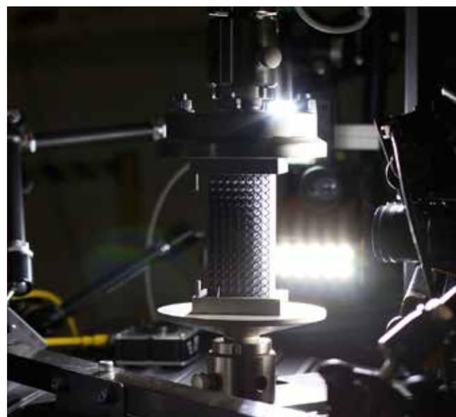
Monitoring by 4 cameras of two faces of a lattice structure during a compression test.
