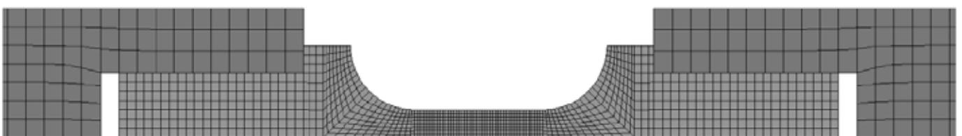
Fig. 4 - 2D axisymmetric FE model for Hopkinson samples.
