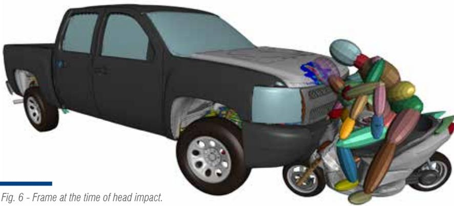
Fig. 6 - Frame at the time of head impact.
