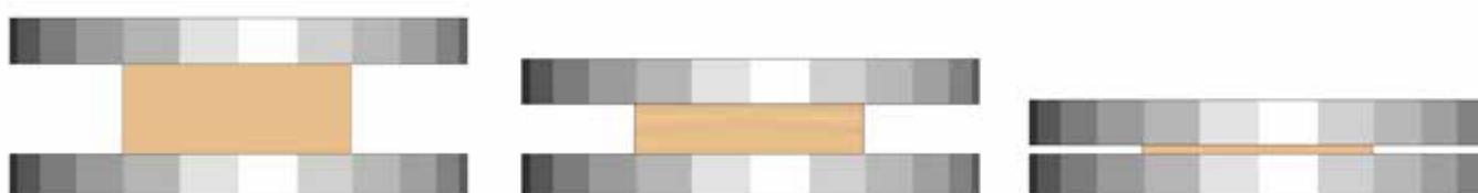
Fig. 6 - Deformation of homogeneous model at different stages.
