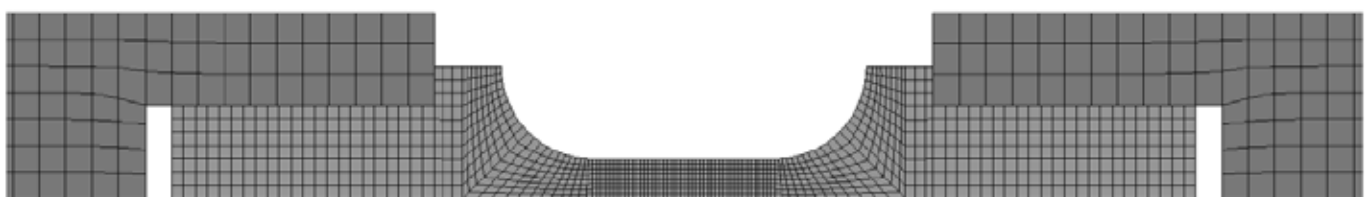
Fig. 4 - 2D axisymmetric FE model for Hopkinson samples.
