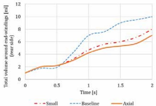
Fig. 11 - Total amount of oil in millilitres around the windings (at the rear of the e-motor). Two proposed bracket designs (Small, Axial) are considered as possible improvements of the baseline.
