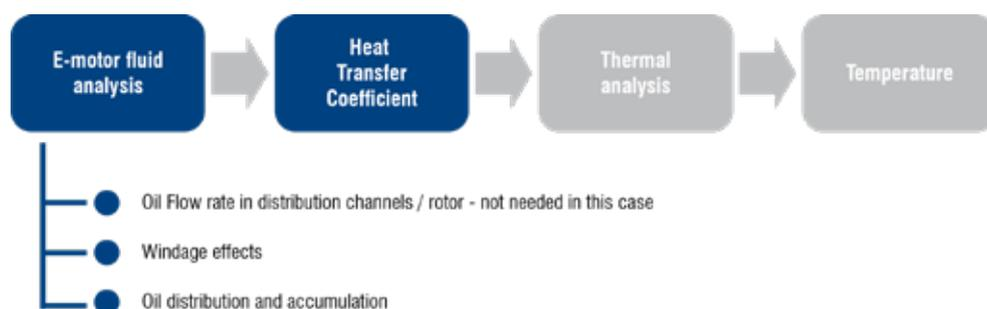
Fig. 1 - Schematic of the simulation methodology for e-motor cooling. The CFD related topics analysed with the MPS method are shown in blue.
