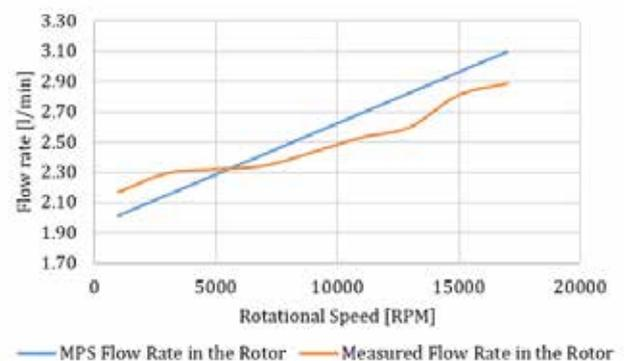
Fig. 5 - Flow rate through the rotor cooling circuit of the out-of-sample dataset (orange) and the predicted trend of the statistical model constructed using the DOE (blue).
