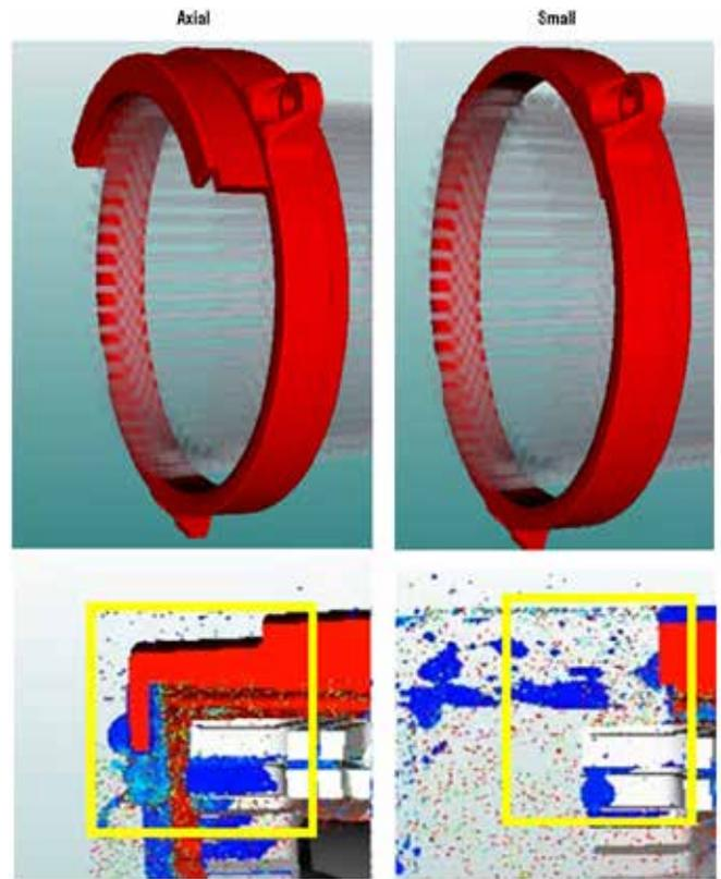
Fig. 10 - Overview of the bracket design (top, isometric view) and detail of the modification near the windings (bottom). As can be seen, the Axial bracket design collects the oil (blue) so it does not splash onto the external housing as seen on the bottom right.
