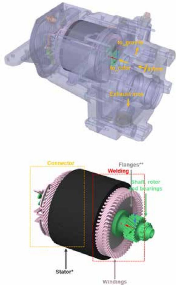
Fig. 2 - Isometric view of the e-motor presented. On the left, the names of the cooling sub-channels. On the right, the names of the most important parts of the e-motor.
