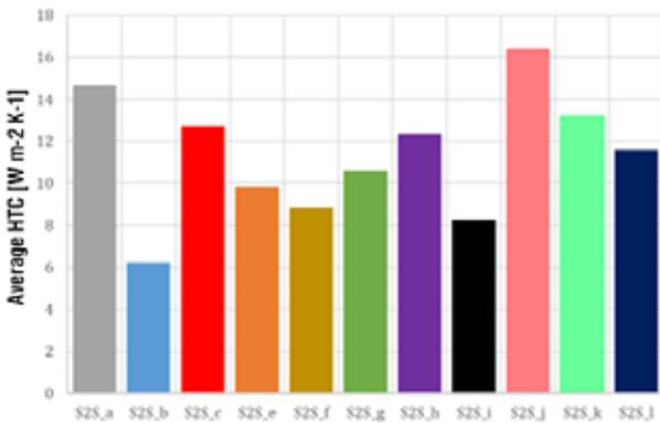
Fig. 8 - Area weighted average HTC across the windings for different flanges (contribution of a single oil jet).
