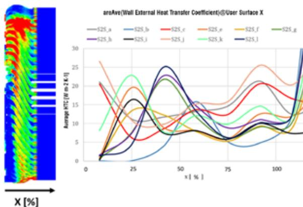
Fig. 9 - AreaAveHTC for different x-slices of the windings. This analysis allows the HTC values to be mapped spatially in a quantitative way.
