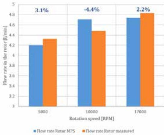
Fig. 6 - Flow rate to the rotor cooling system (rotor circuit) for three rotor speeds. The MPS predictions (blue) are compared to the experimental results (orange).
