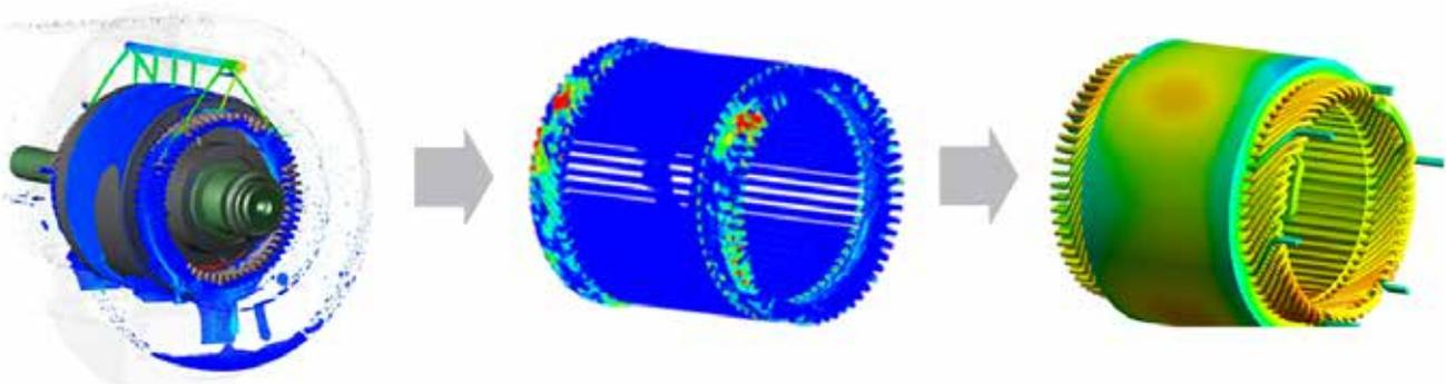
Fig. 4 - From oil distribution to temperature distribution. On the left, the oil can be inspected and, once stabilized, an HTC map is extracted. The maps are transferred to the FEA model to obtain the temperature prediction.
