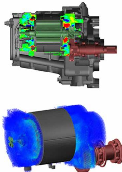
Fig. 3 - Overview of the airfield as calculated by the MPS method (top) and the same airfield as imported into the oil-only simulation (bottom).
