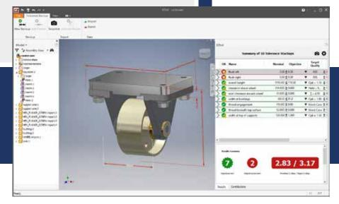
EZtol is a 1-Dimensional tolerance stackup analysis program designed to assist in understanding the impact of part-level dimensional variation accumulation, part-to-part assembly variation sources and the consequential impact that they have on assembly-level requirements.
