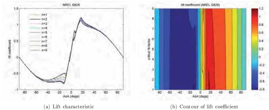
Figure 8. Effect of critical N-factor on NREL S828 cross-section.  $Re=1015166.4253$ ,  $M=0.1218$ .
