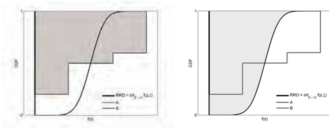
(a) The shaded area is the RI for candidate design A (b) The shaded area is the RI for candidate design B
