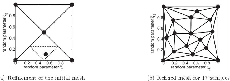
Figure 2. Simplex Stochastic Collocation discretization of a two-dimensional probability space.
