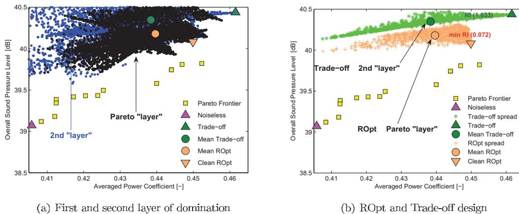
Figure 11. Probabilistic Pareto front [detail]
