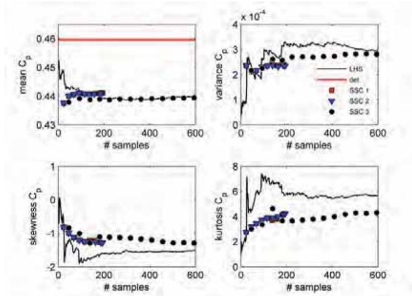
Figure 9. Analysis under uncertainty due to Insect contamination: convergence histories of the mean, variance, skewness and kurtosis of the power coefficient
