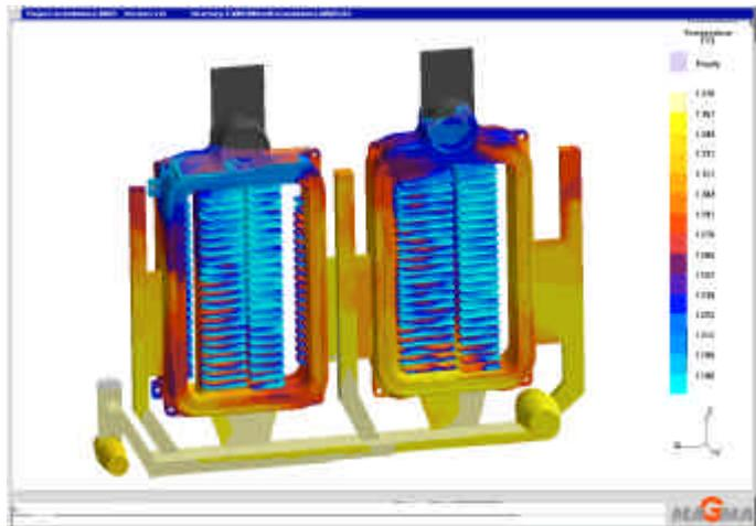
*Fig. 12 – Temperature distribution during filling simulation*
