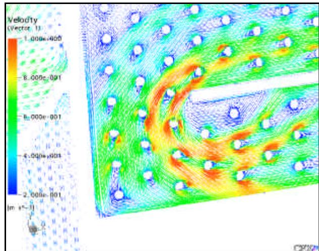
Fig. 4 – Flow path around the pins
