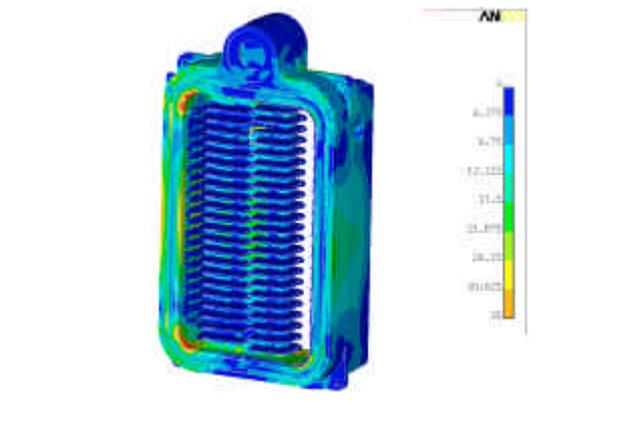
Fig. 16 – Residual Von Mises stress transferred in ANSYS
