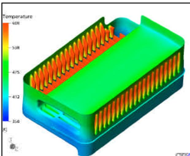
Fig. 5 – Temperature distribution of grey iron surface
