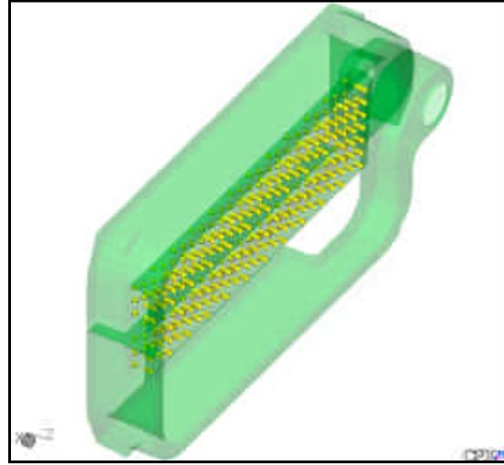
Fig. 1 – Heat transfer surface between Iron and Water      Fig.2 – Mesh of central chamber and pins
