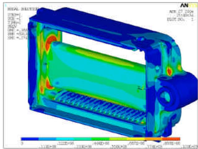
Fig. 8 – Von Mises equiv. stress
