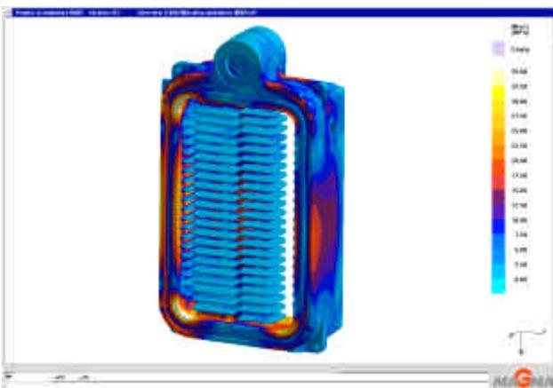
Fig. 15 – Residual Von Mises stress in MAGMASOFT
