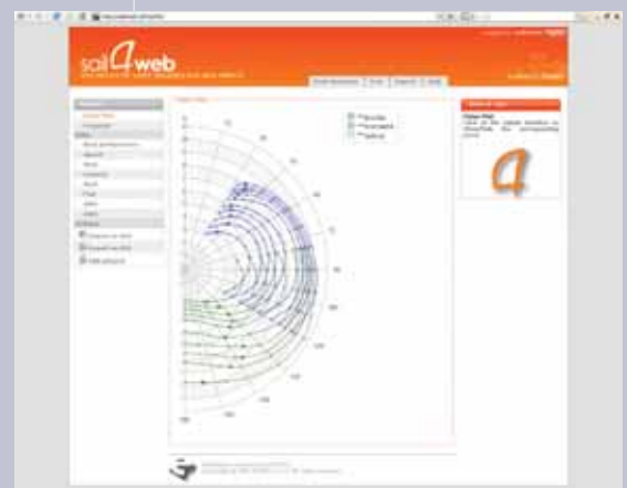
Figure 7: Sail4web screenshot – VPP polar plot
