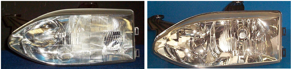
Figure 1: comparison between an old fashioned glass headlamp (left) and a new transparent plastic headlamp (right)
